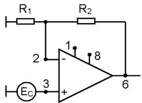
$$\frac{R_2}{R_1} \geq 19 \quad K_y \geq 20$$
