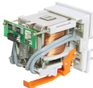
**Application of electronics made in the SMD technology:** additional features L (LED diode) and D (diode) are located on the printed circuit board; the change of the position of the LED diode and optimization of the quality and intensity of its light provide certainty that the relay is in operation status when the LED is on.
