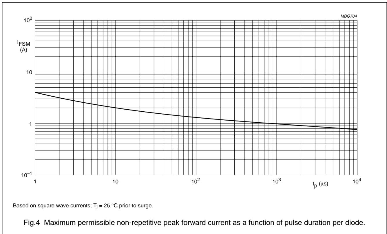
Low-leakage double diode
