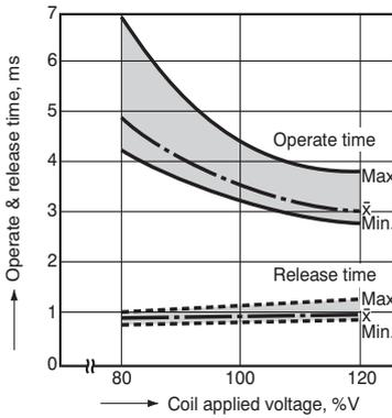
4.-(2) Operate & release time (without diode, 1 Form A 1 Form B)
