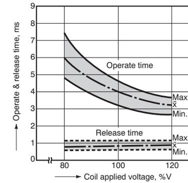
4.-(4) Operate & release time (with diode, 1 Form A)
