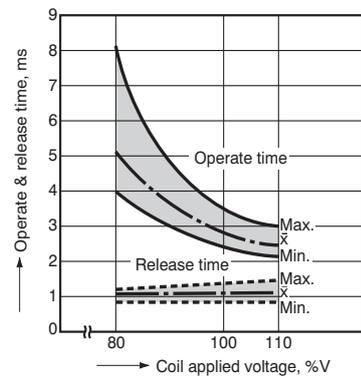
4.-(3) Operate & release time (without diode, 2 Form A)
