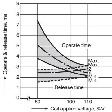
4.-(6) Operate & release time (with diode, 2 Form A)
