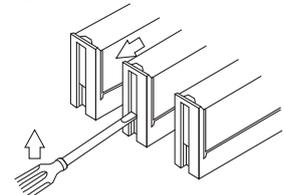
Notes: 1. Exercise care when removing relays. If greater than necessary force is applied at the socket hooks, deformation may alter the dimensions so that the hook will no longer catch, and other damage may also occur.
