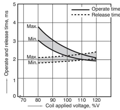
6-(2). Operate and release time (without diode)
