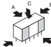
Please chuck the
