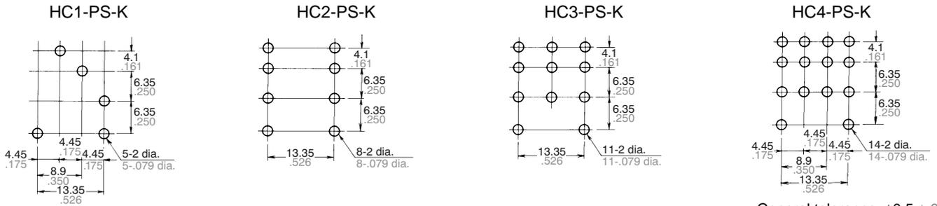
**Screw socket mounts (Top view)**
