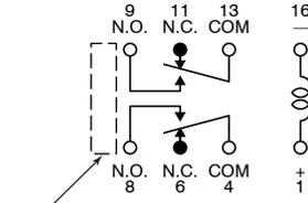
\*A polarity bar shows the relay direction.
