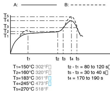
Temperature rise of relay itself may vary according to the mounting level or the heating method of reflow equipment. Therefore, please set the temperature of soldering portion of relay terminal and the top surface of the relay case not to exceed the above mentioned soldering condition.
