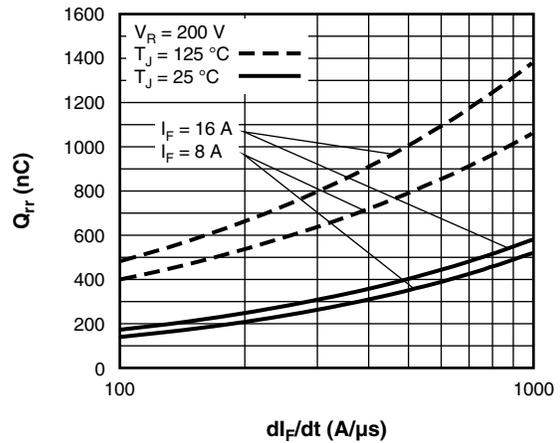
Fig. 7 - Typical Stored Charge vs.  $di_F/dt$  (Per Leg)
