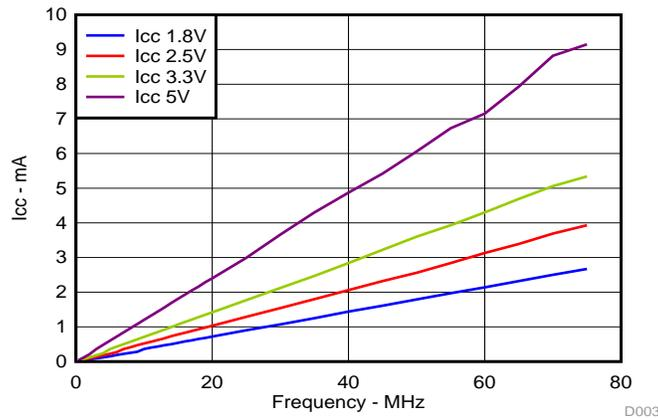
Figure 6. I<sub>CC</sub> vs Frequency
