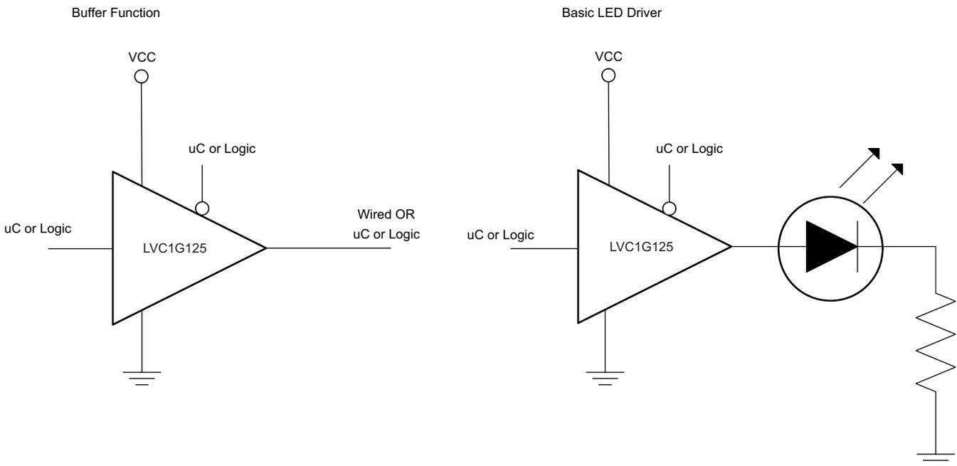
**Figure 5. Application Schematic**
