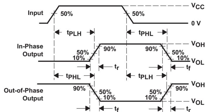
Figure 3. Propagation Delay and Output Transition Times
