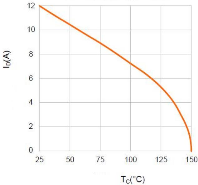
Figure10. Maximum Continuous Drain Current vs Case Temperature
