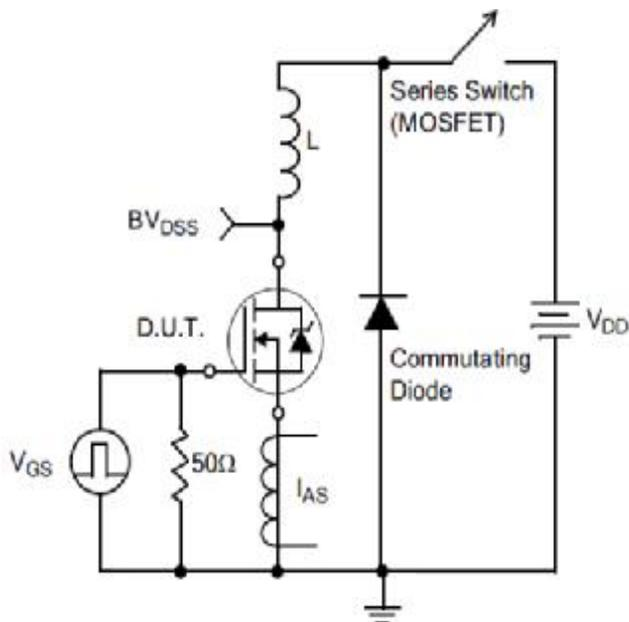
Figure17. Unclamped Inductive Switching Test Circuit
