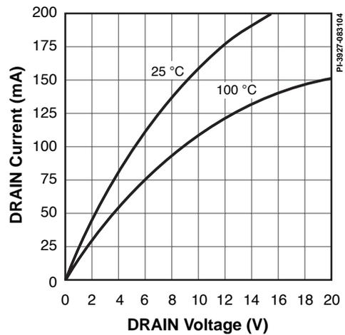
Figure 16. Output Characteristics.
