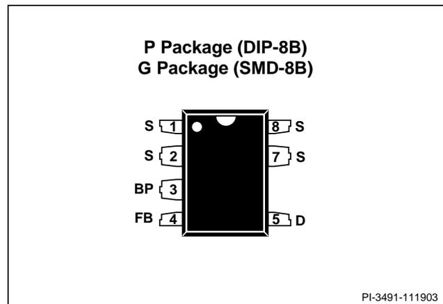
Figure 3. Pin Configuration.
