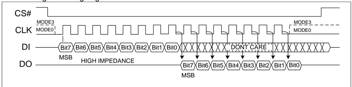
Figure 2 The difference between Mode 0 and Mode 3
