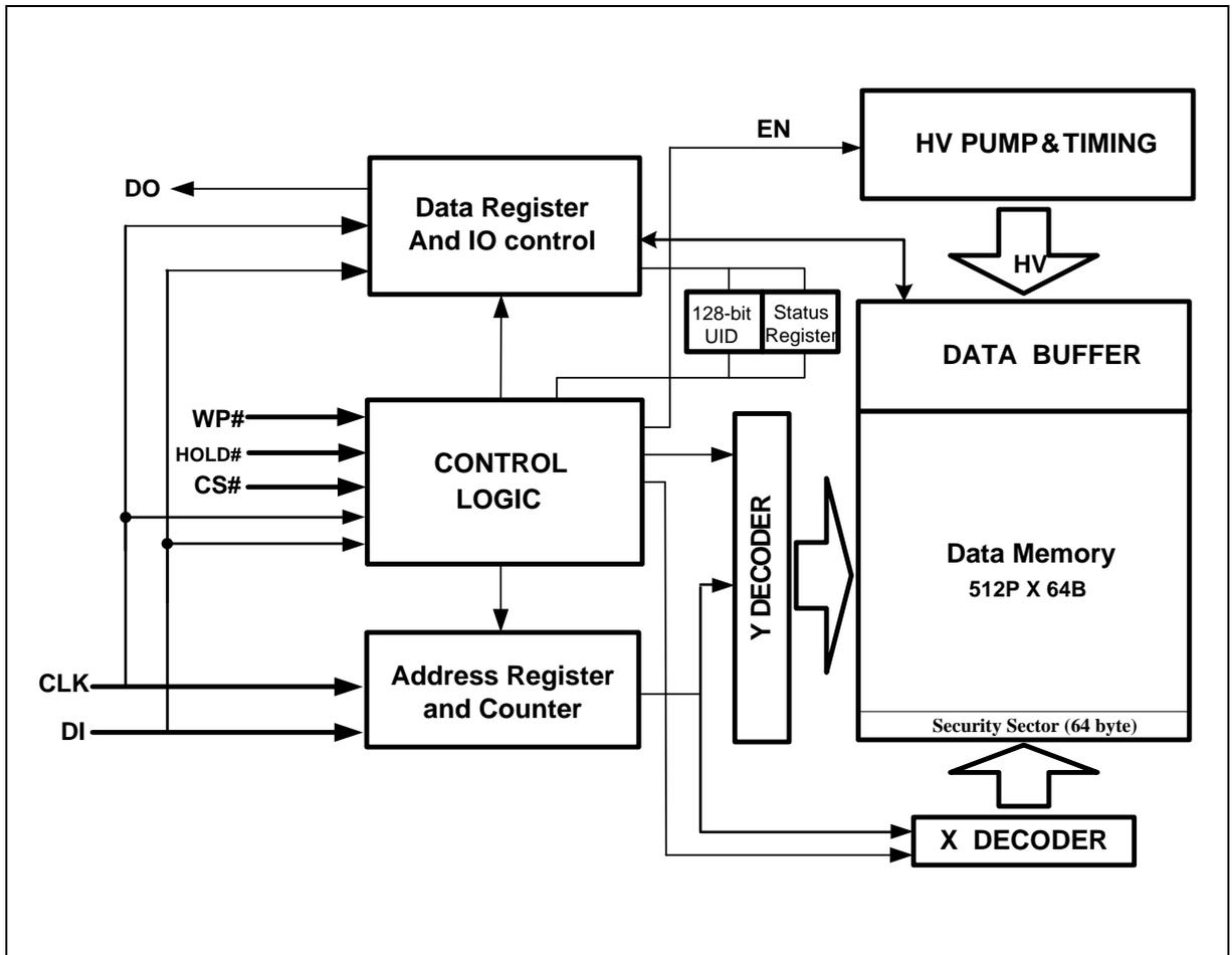
Figure 1 Block Diagram
