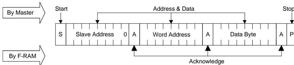
Figure 8. Multi-Byte Write
