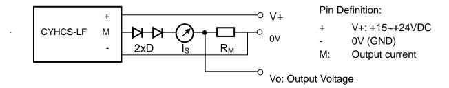
Two diodes for instance IN4007 must be connected at the output of the sensor in order to guarantee the sensor to work well.
