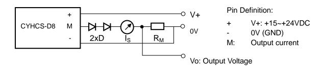
Two diodes for instance IN4007 must be connected at the output of the sensor in order to guarantee the sensor to work well.
