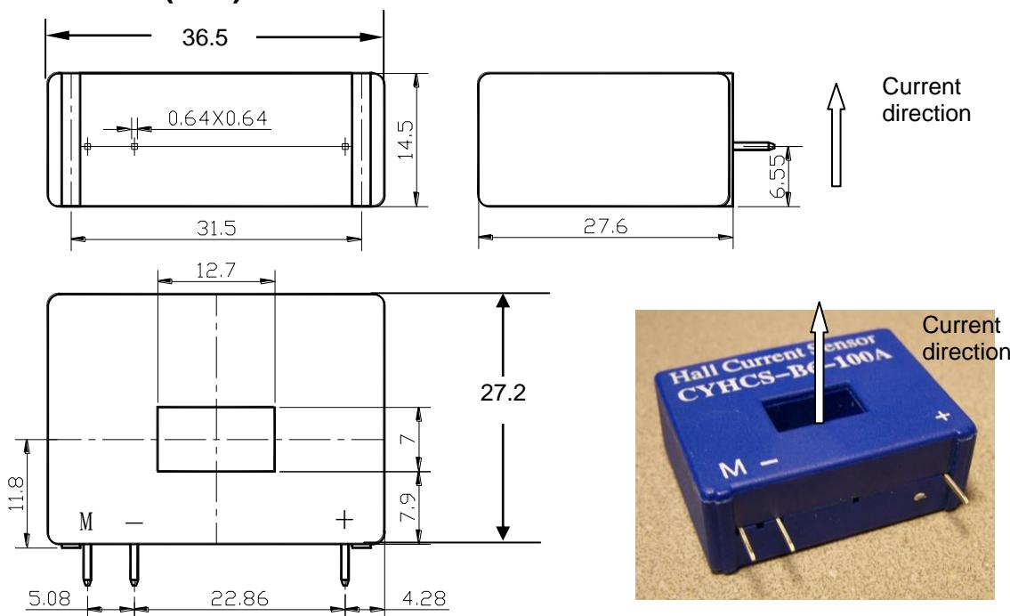
Terminal +: +12V~ 15V, Terminal -: -12V~ -15V, Terminal M: Output
