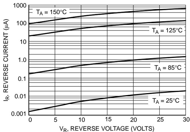
**Figure 3. Leakage Current**
