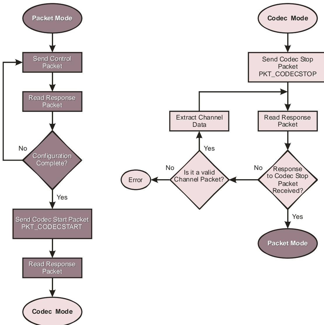
Figure 19 Switching between Packet and Codec Modes
