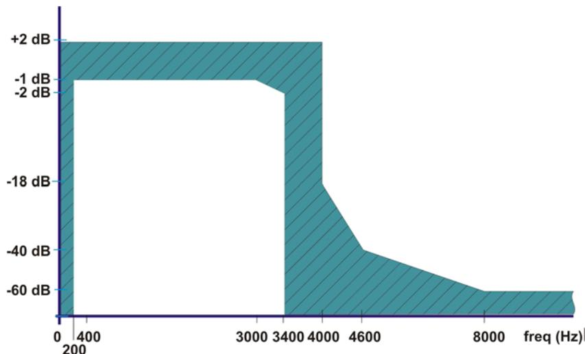
Figure 38 Front End Output Filter Mask
