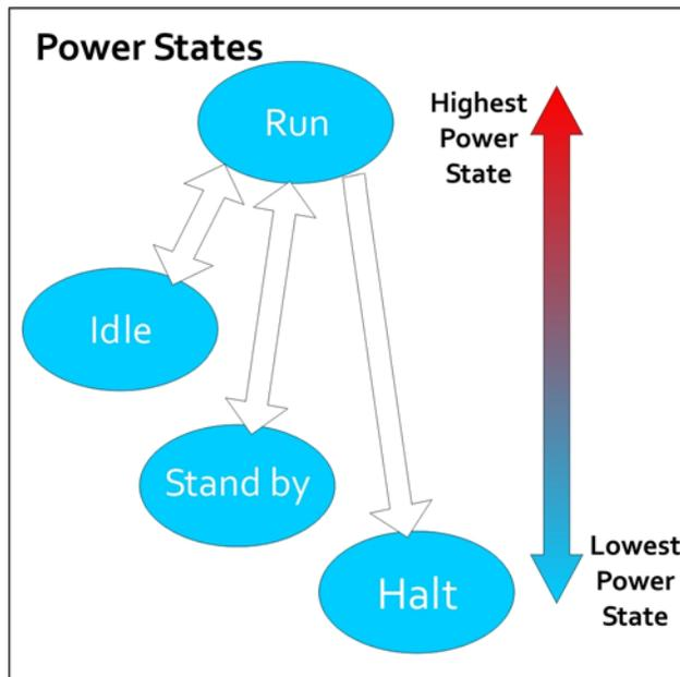
Figure 14 AMBE-3000F™ Vocoder Chip Power States
