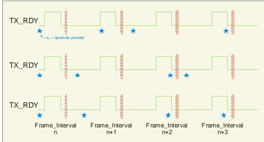
**Figure 26 TX\_RDY Frame interval Examples**
