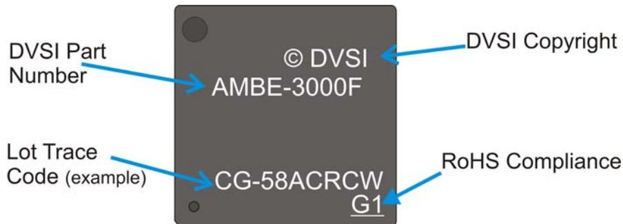
Figure 6 AMBE-3000F™ Vocoder Chip Markings for BGA
