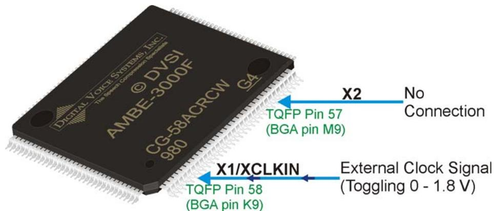
Figure 7 X1/XCLKIN and X2 with TTL/CMOS Clock Source
