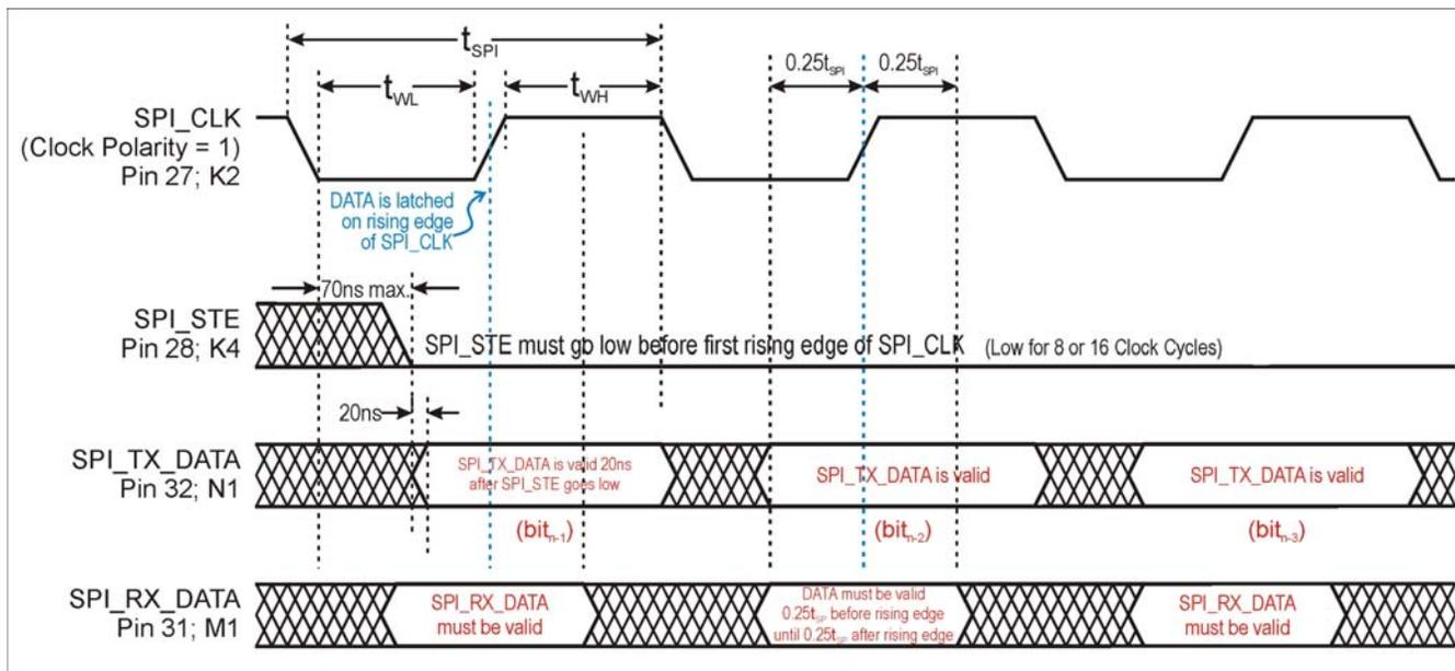
Figure 30 SPI Timing
