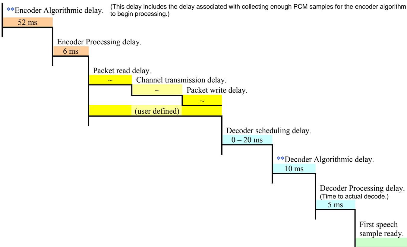
**\*\*Note:** The total algorithmic delay for the encoder and decoder combined is 62 msec. The breakdown in this chart is somewhat arbitrary but it represents a close estimate.
