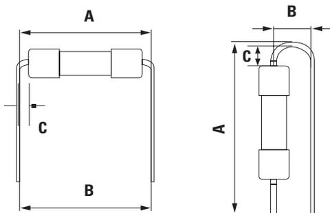
For the pigtailed fuse, please follow the recommendations below for axial lead forming and mounting into PCB:
