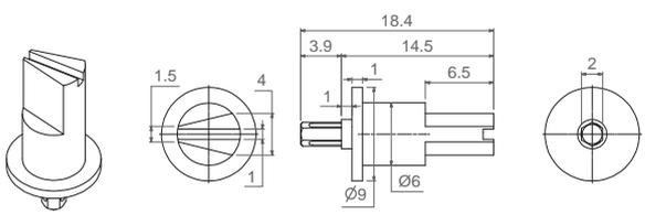
The arrow is in line with the wiper when potentiometer has rotor J (with M rotor, there is a 30° difference).
