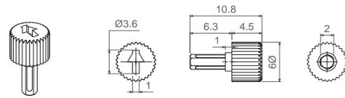
The arrow is in line with the wiper when potentiometer has rotor J (with M rotor, there is a 30° difference).
