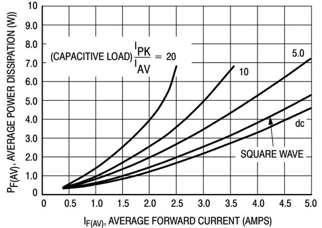
Figure 3. Power Dissipation
