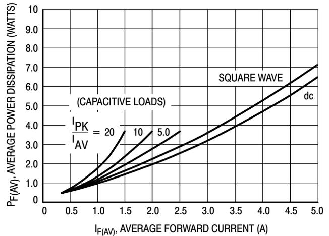
Figure 8. Power Dissipation
