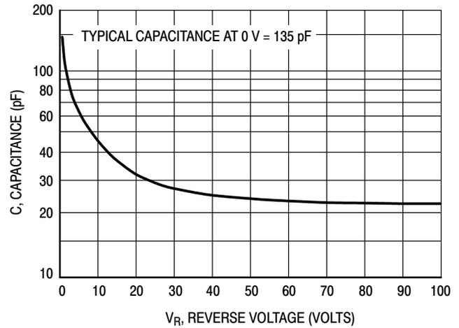
Figure 5. Typical Capacitance
