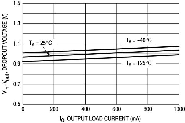
Figure 2. Dropout Voltage versus Output Load Current
