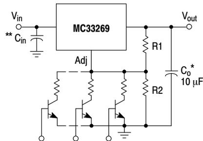
R<sub>2</sub> sets the maximum output voltage. Each transistor reduces the output voltage when turned on.
