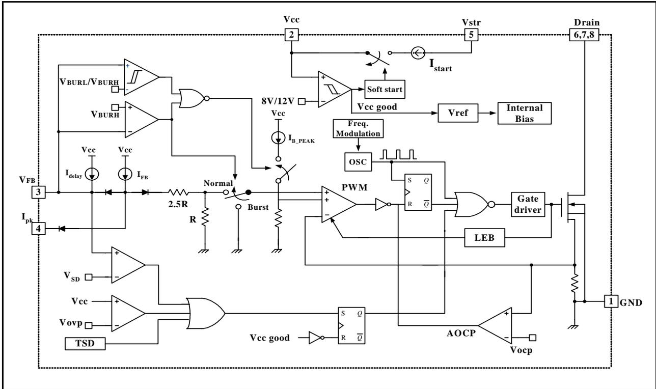
Figure 2. Functional Block Diagram of FSDx321
