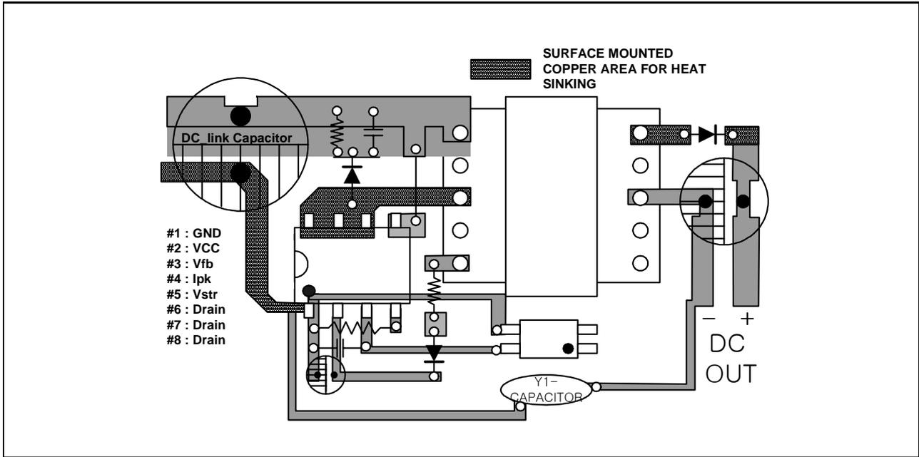
Figure 13. Layout Considerations for FSDx321 using 8DIP
