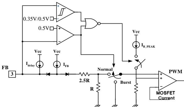
Figure 9. Circuit for Burst operation
