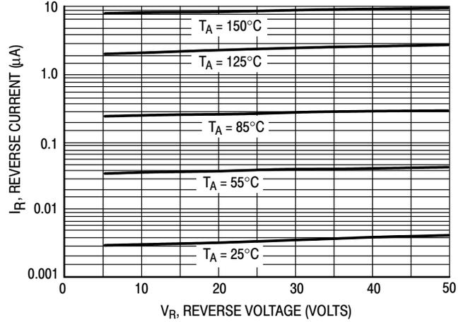
Figure 3. Leakage Current
