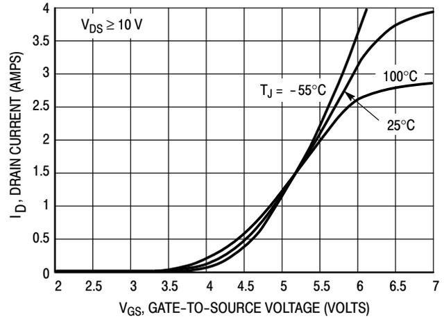
Figure 2. Transfer Characteristics
