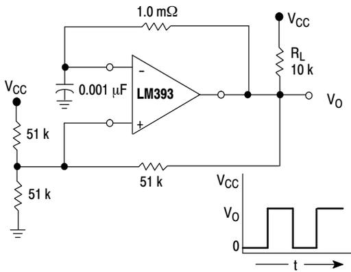
Figure 10. Free-Running Square-Wave Oscillator
