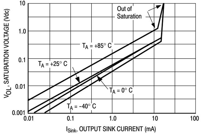
Figure 5. Output Saturation Voltage versus Output Sink Current
