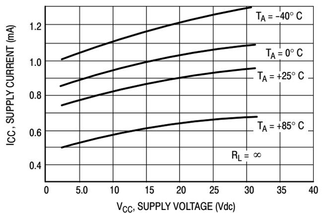
Figure 7. Power Supply Current versus Power Supply Voltage
