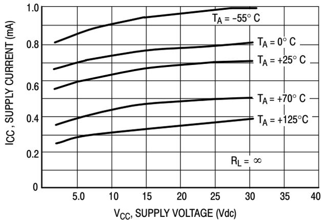
Figure 6. Power Supply Current versus Power Supply Voltage
