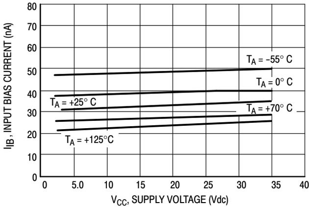
Figure 2. Input Bias Current versus Power Supply Voltage
