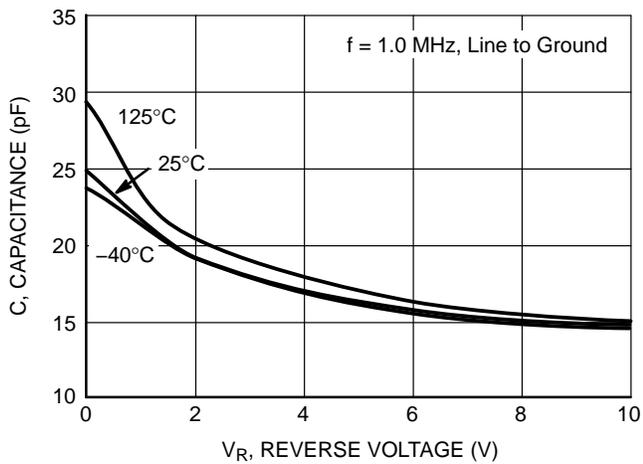
Figure 3. Typical Junction Capacitance vs Reverse Voltage
