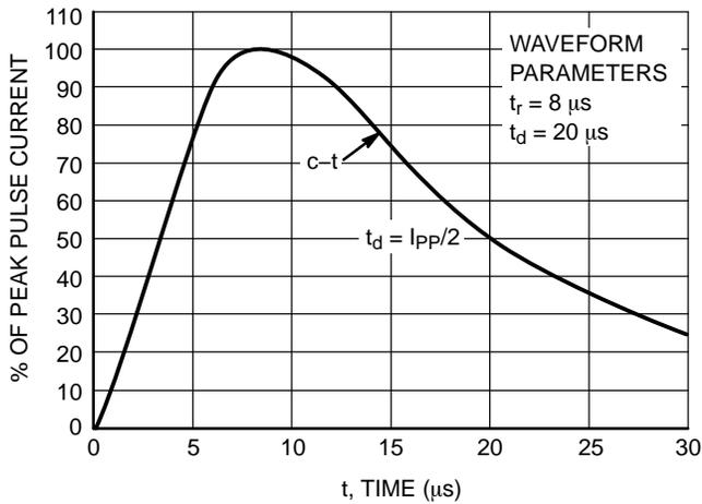
Figure 1. Pulse Waveform, IEC 61000-4-5 8/20  $\mu\text{s}$
