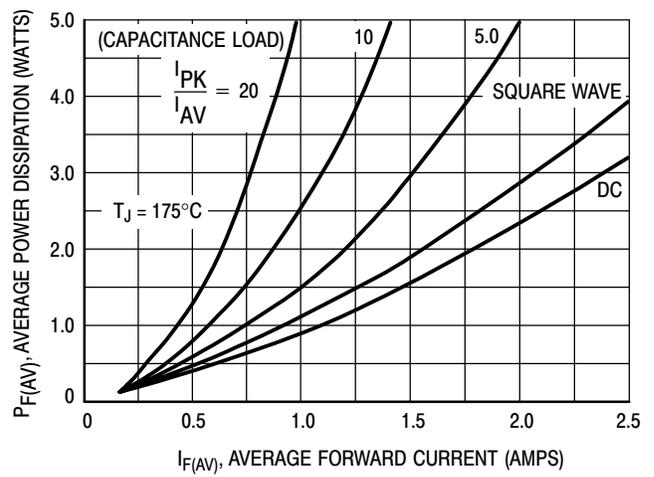
Figure 10. Power Dissipation
