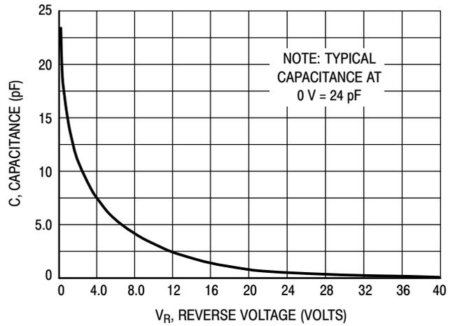
Figure 8. Typical Capacitance
