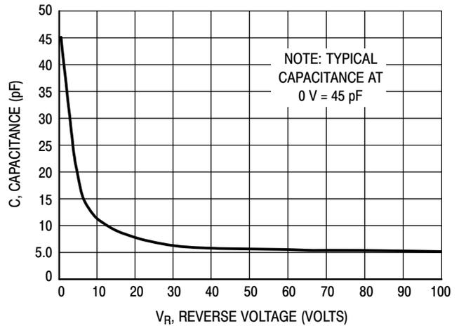
Figure 3. Typical Capacitance
