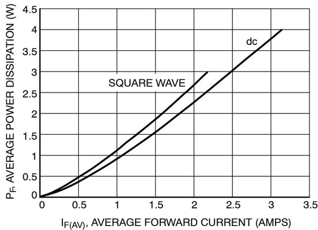
Figure 9. Power Dissipation
