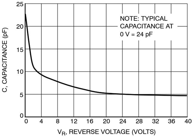
Figure 5. Typical Capacitance
