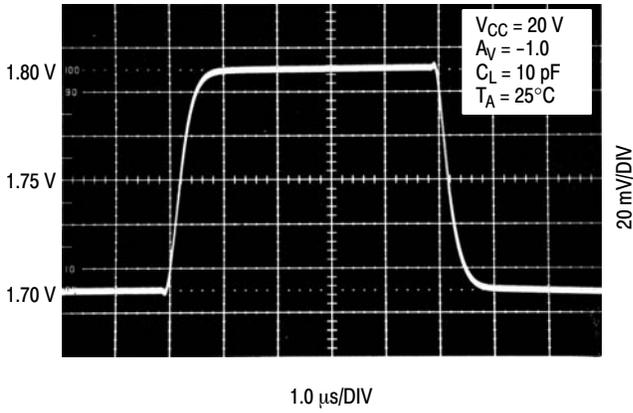
Figure 8. Error Amplifier Small Signal Transient Response
