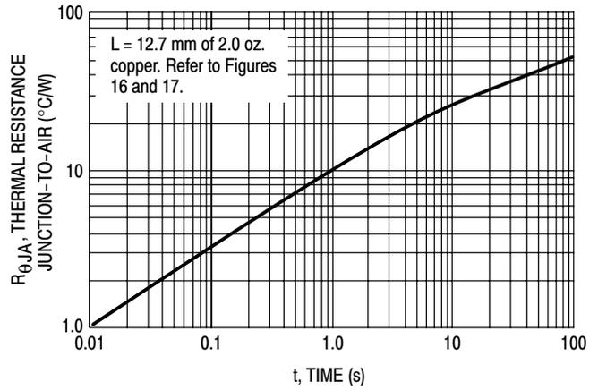
Figure 15. DW and P Suffix Transient Thermal Resistance
