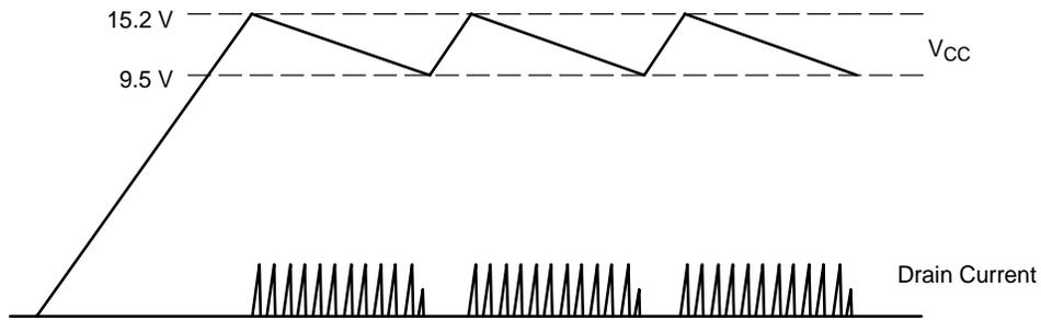
Figure 20. Timing Diagram of Short-Circuit Condition
