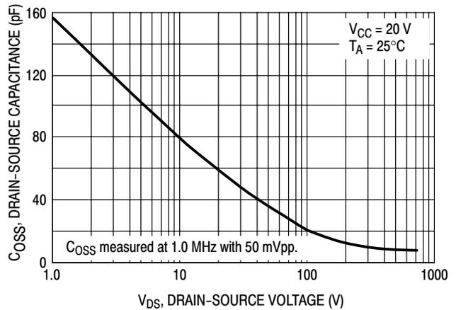
Figure 13. Power Switch Drain-Source Capacitance versus Voltage
