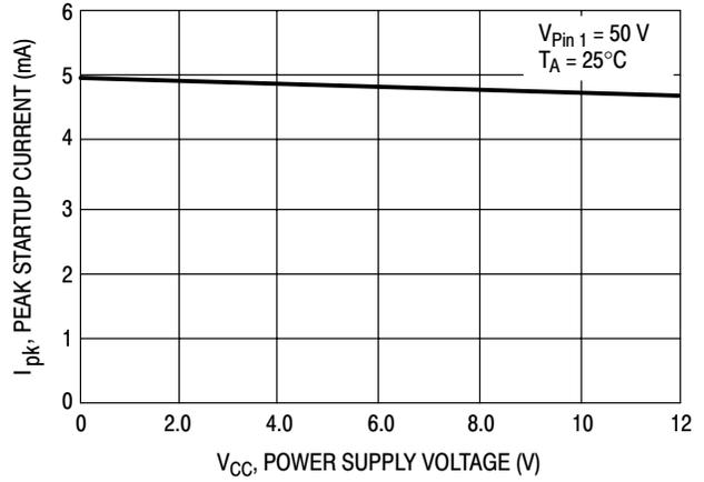
Figure 11. Peak Startup Current versus Power Supply Voltage
