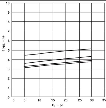
$T_A = 25^\circ\text{C}, V_{CCA} = 5\text{ V}$
