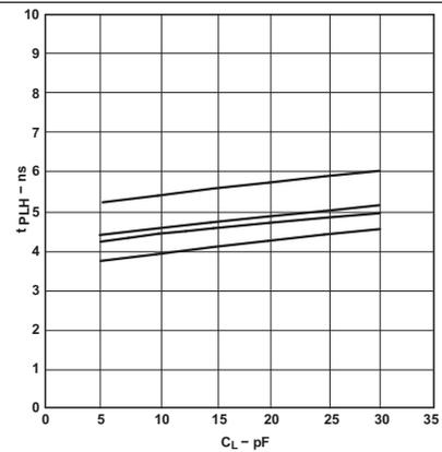
$T_A = 25^\circ\text{C}, V_{CCA} = 5\text{ V}$
