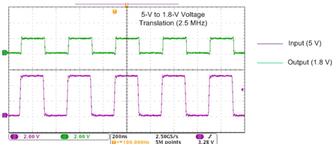
Figure 14. Translation Down (5V to 1.8 V) at 2.5 MHz
