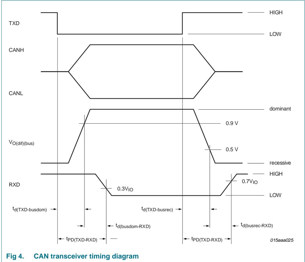
Fig 4. CAN transceiver timing diagram
