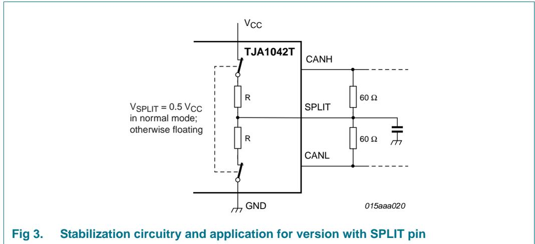
Fig 3. Stabilization circuitry and application for version with SPLIT pin
