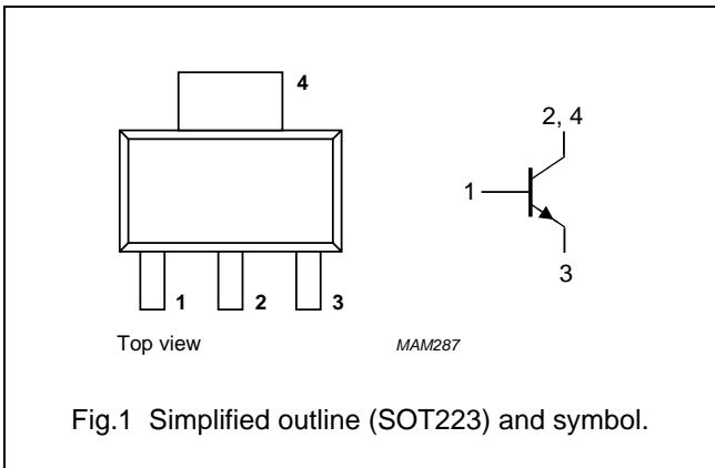
40 V low  $V_{CEsat}$  NPN transistor
