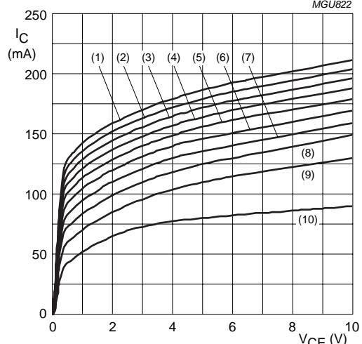
Fig.3 Collector current as a function of collector-emitter voltage.
