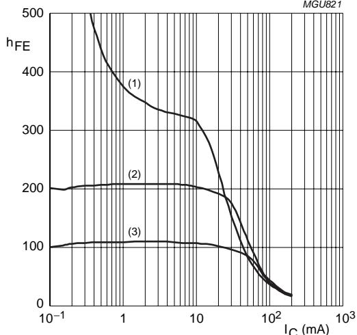
Fig.2 DC current gain; typical values.
