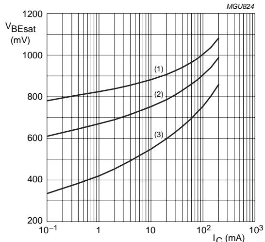
Fig.5 Base-emitter saturation voltage as a function of collector current.
