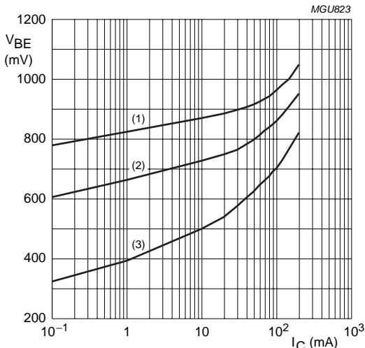
Fig.4 Base-emitter voltage as a function of collector current.
