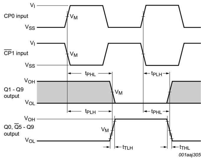
Conditions:  $\overline{CP1} = \text{LOW}$ , while CP0 triggers on a LOW-to-HIGH transition.  $\overline{CP1}$  triggers on a HIGH-to-LOW transition;
