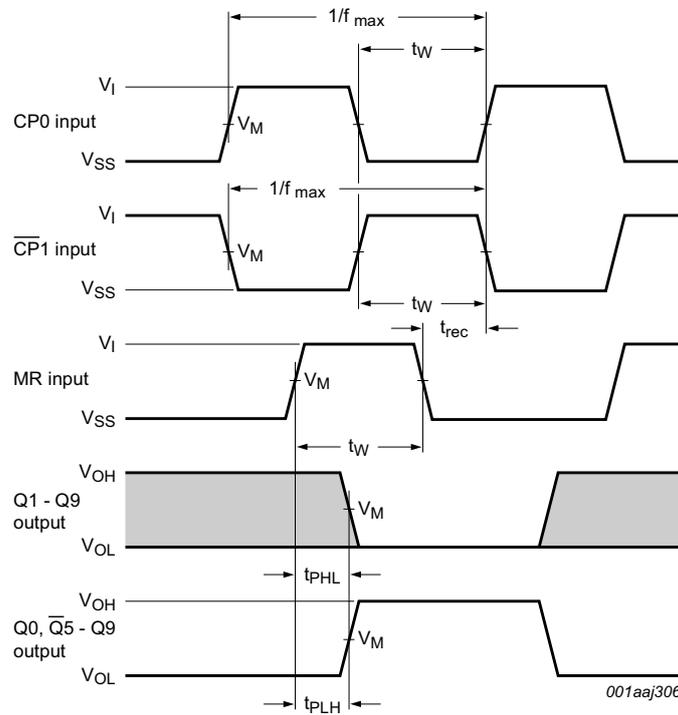
Conditions:  $\overline{CP1} = \text{LOW}$ , while CP0 triggers on a LOW-to-HIGH transition,  $t_W$  and  $t_{rec}$  are measured when CP0 = HIGH and  $\overline{CP1}$  triggers on a HIGH-to-LOW transition.
