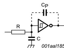
Fig 11. Schmitt trigger driven via a high-impedance input
