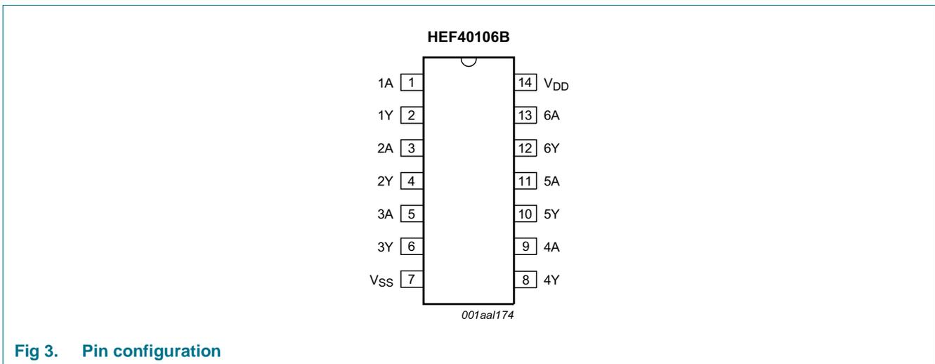
Fig 3. Pin configuration
