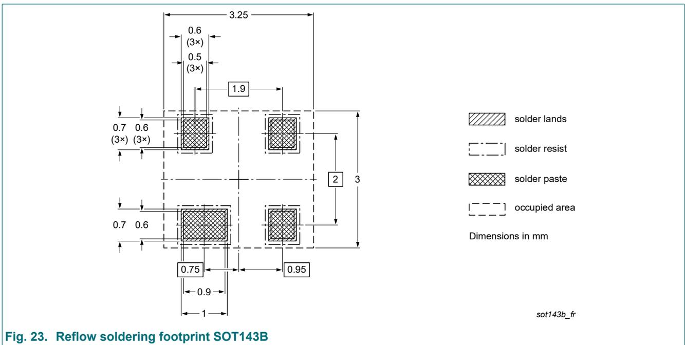
Fig. 23. Reflow soldering footprint SOT143B
