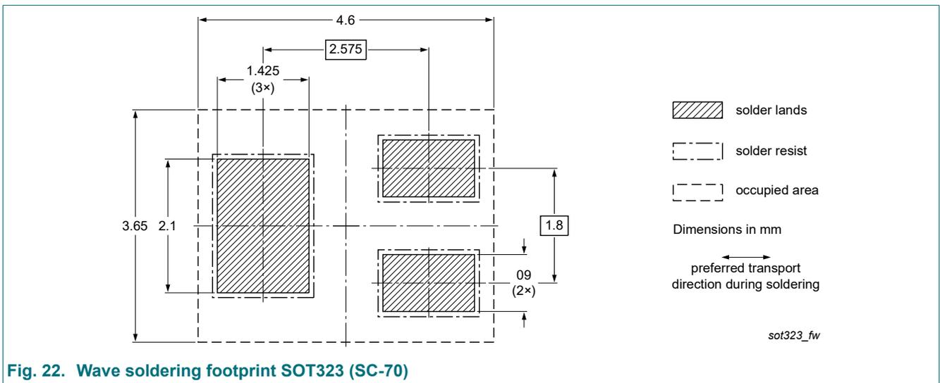
Fig. 22. Wave soldering footprint SOT323 (SC-70)
