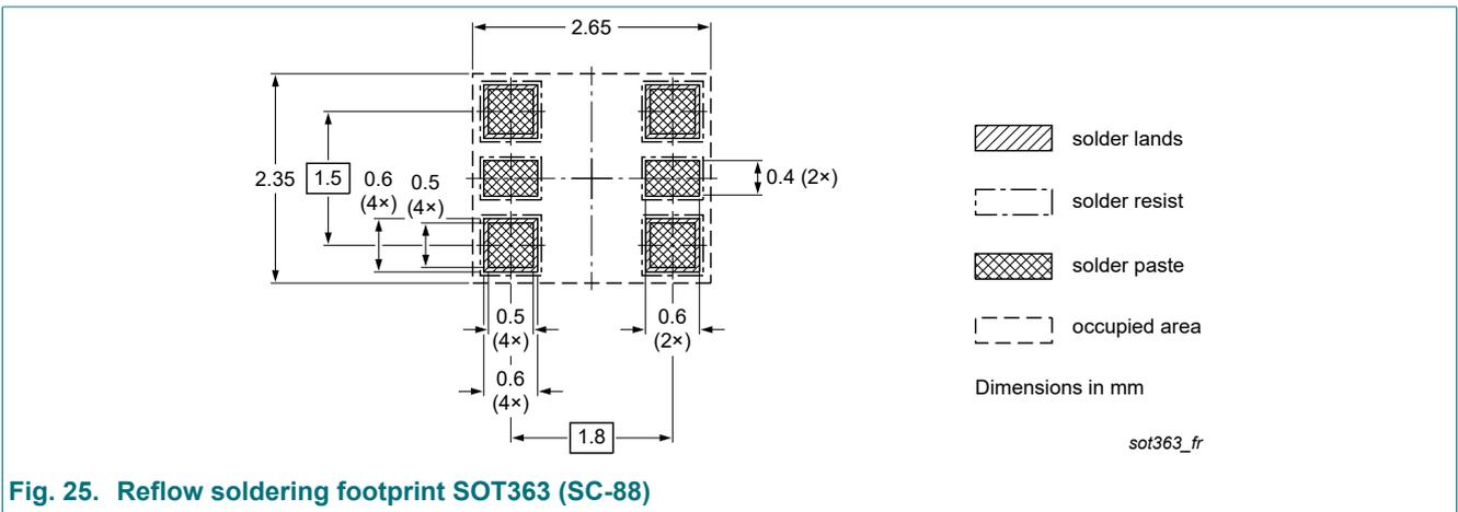
Fig. 25. Reflow soldering footprint SOT363 (SC-88)
