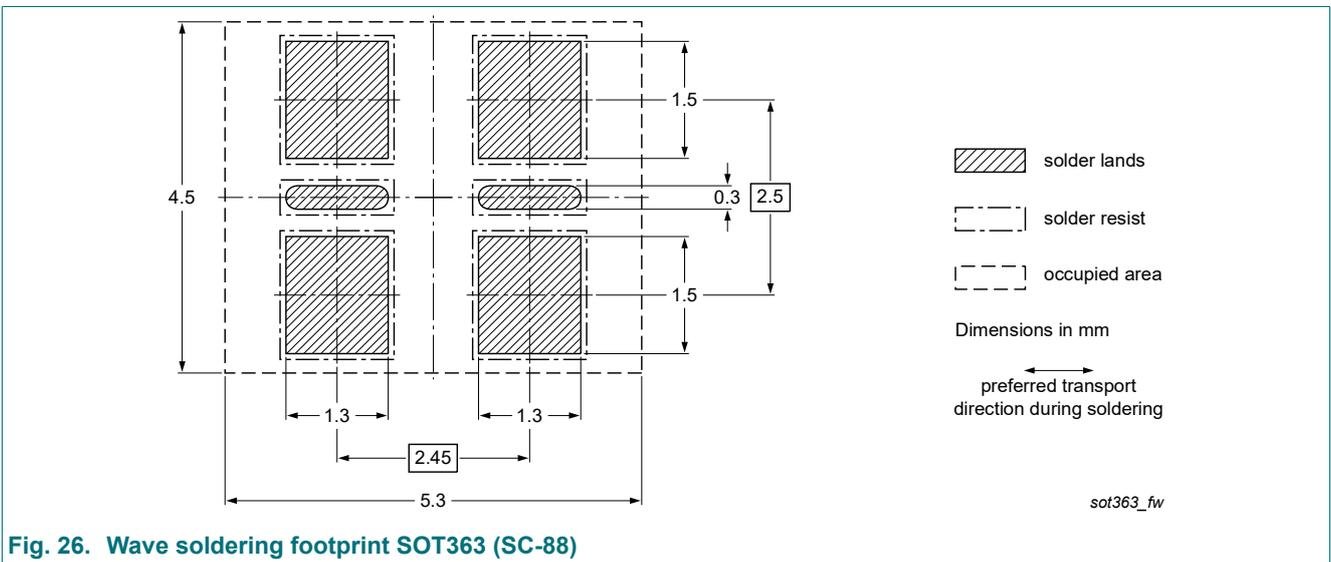
Fig. 26. Wave soldering footprint SOT363 (SC-88)
