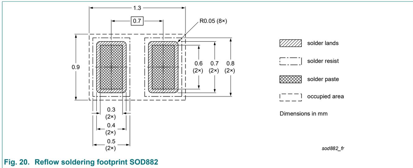
Fig. 20. Reflow soldering footprint SOD882
