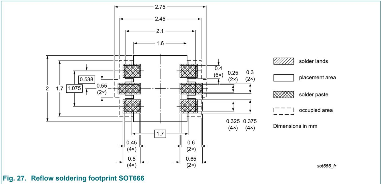
Fig. 27. Reflow soldering footprint SOT666
