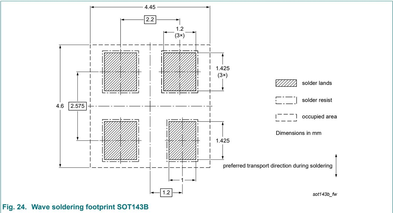
Fig. 24. Wave soldering footprint SOT143B
