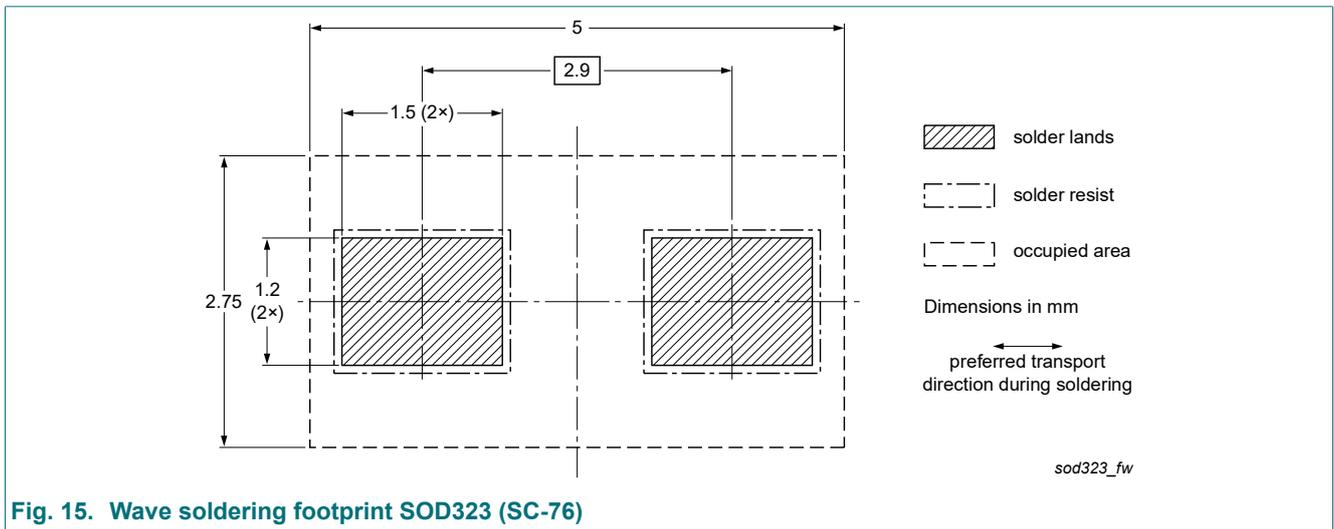
Fig. 15. Wave soldering footprint SOD323 (SC-76)
