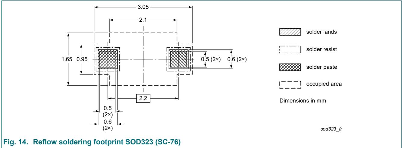
Fig. 14. Reflow soldering footprint SOD323 (SC-76)
