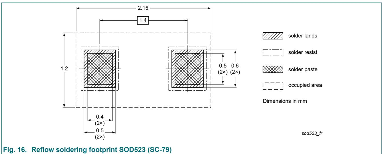
Fig. 16. Reflow soldering footprint SOD523 (SC-79)
