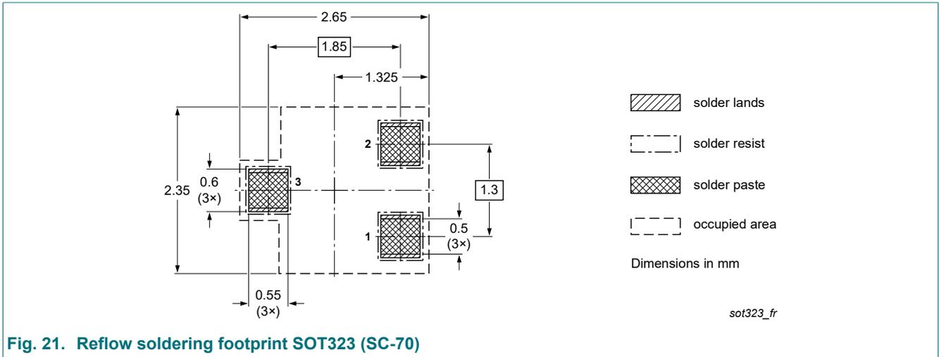
Fig. 21. Reflow soldering footprint SOT323 (SC-70)
