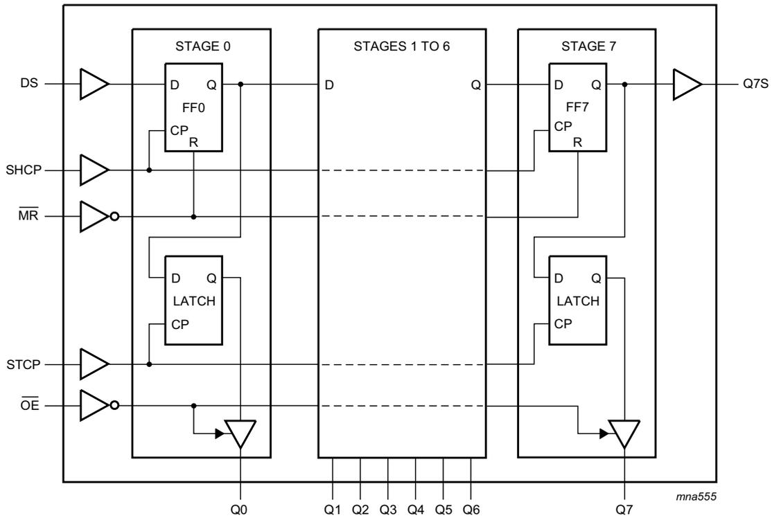
Fig 4. Logic diagram
