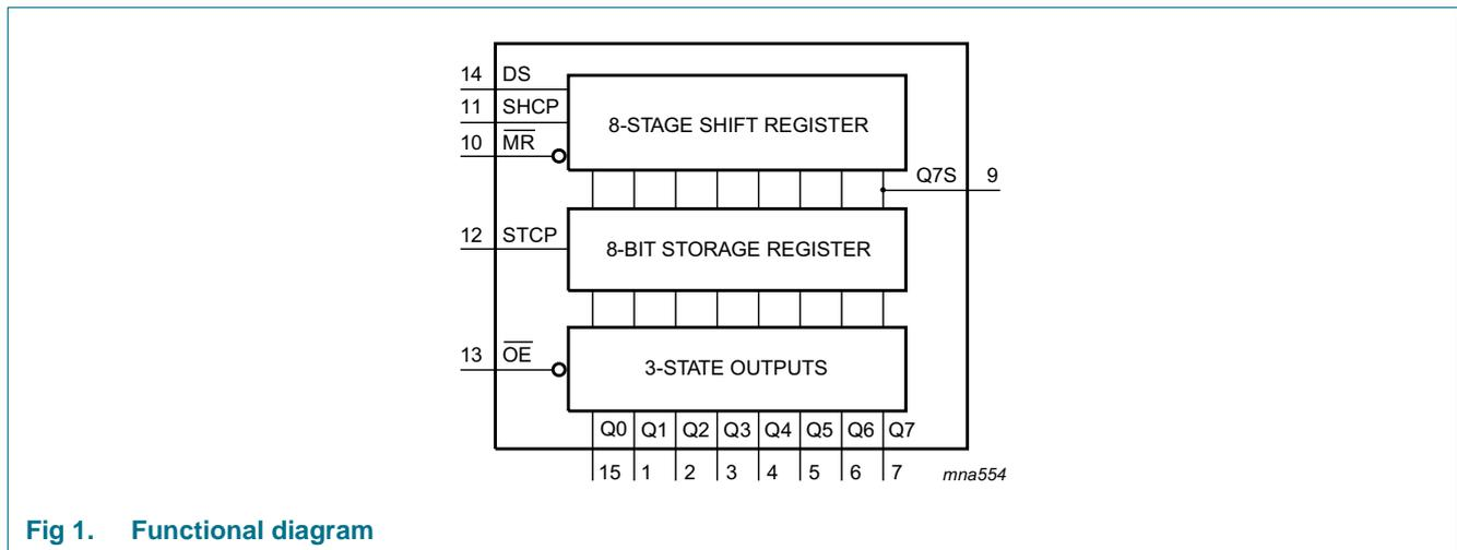
Fig 1. Functional diagram
