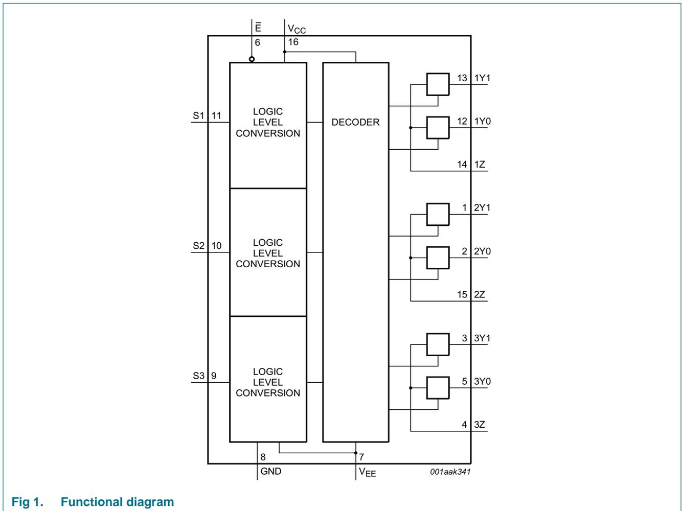
Fig 1. Functional diagram
