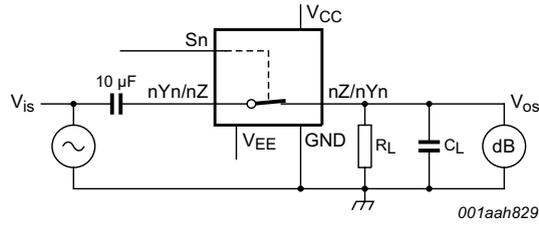
Fig 16. Test circuit for measuring sine-wave distortion
