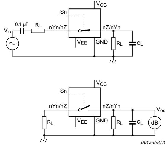
Fig 18. Test circuits for measuring crosstalk between any two switches/multiplexers
