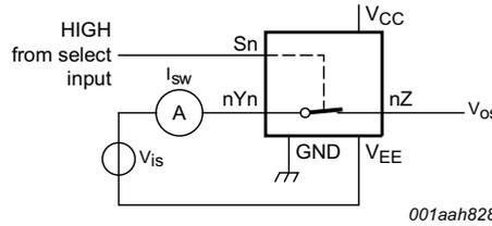
$V_{is} = V_{CC}$  and  $V_{os} = \text{open-circuit}$ .
