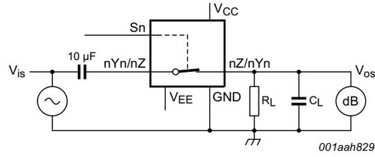
$V_{CC} = 4.5 \text{ V}$ ;  $GND = 0 \text{ V}$ ;  $V_{EE} = -4.5 \text{ V}$ ;  $R_L = 50 \text{ } \Omega$ ;  $R_S = 1 \text{ k}\Omega$ .
