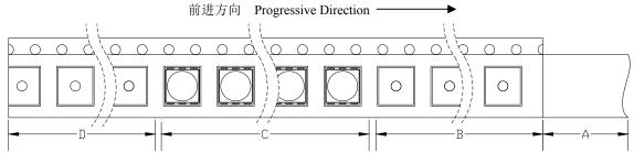
A: 盖带, 300 mm; B: 引导, 空带, 200mm; C: 编载产品 3500 只; D: 尾部, 空带, 200mm A: Top Cover Tape, 300mm; B: Leader, Empty, 200mm; C: 3500 Lamps Loaded; D: Trailer, Empty, 200mm.
