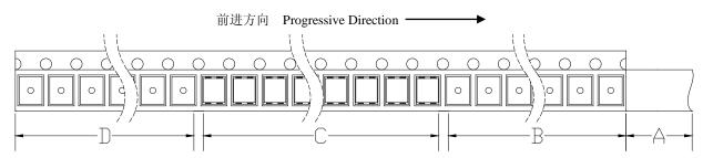
A: 盖带, 300 mm; B: 引导, 空带, 200mm; C: 编载产品 800 只; D: 尾部, 空带, 200mm A: Top Cover Tape, 300mm; B: Leader, Empty, 200mm; C: 800 Lamps Loaded; D: Trailer, Empty, 200mm.
