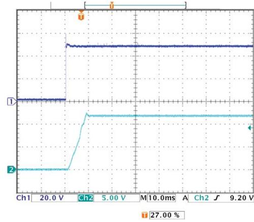
Start-up Parallel Operation (Vin=48V, Iout=full load, Cload=10000µF, Ta=+25°C) Ch1= Vin, Ch2, Ch3= Vout
