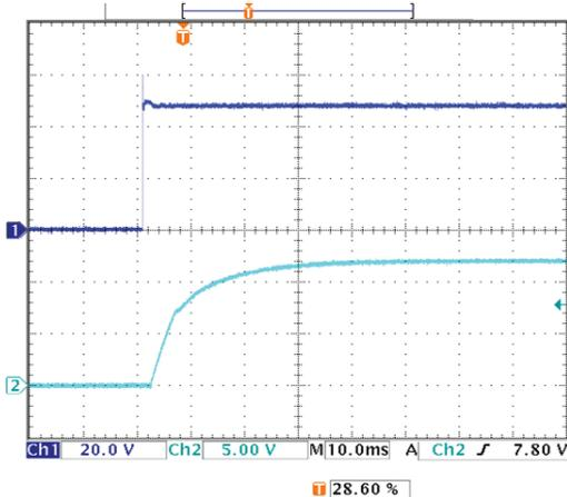
On/Off Enable Delay (Vin=48V, Vout=nom, Iout=20A, Cload=5000μF, Ta=+25°C)
