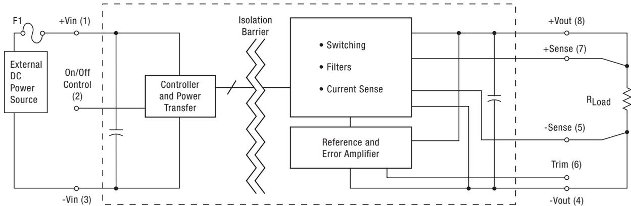
Figure 1. Connection Diagram
