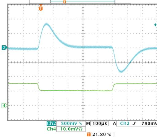
Output ripple and Noise (Vin=48V, Iout=0A, Cload= 1μF || 10μF, Ta=+25°C, BW=20Mhz)
