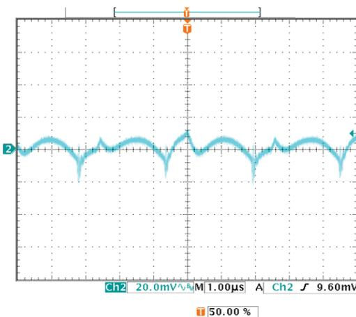
Output ripple and Noise (Vin=48V, Iout=20A, Cload= 1μF || 10μF, Ta=+25°C, BW=20Mhz)
