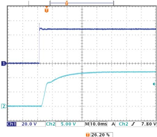
Start-up Delay (Vin=48V, Iout=20A, Cload=5000μF, Ta=+25°C) Ch1= Vin, Ch2= Vout
