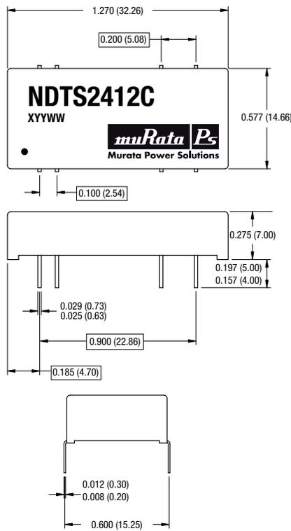
All dimensions in inches  $\pm 0.01$  (mm  $\pm 0.25$ mm). All pins on a 0.1 (2.54) pitch and within  $\pm 0.01$  (0.25) of true position. Weight: 6.2g
