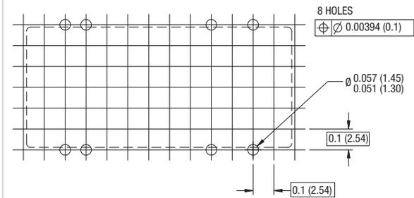
All dimensions in inches  $\pm 0.01$  (mm  $\pm 0.25$ mm). All pins on a 0.1 (2.54) pitch and within  $\pm 0.01$  (0.25) of true position.
