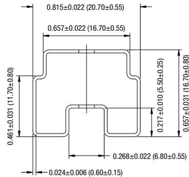
All dimensions in inches  $\pm 0.01$  (mm)  $\pm 0.5$ mm. Tube length : 20.47 $\pm$ 0.079 (520mm  $\pm$ 2mm). Tube Quantity : 15
