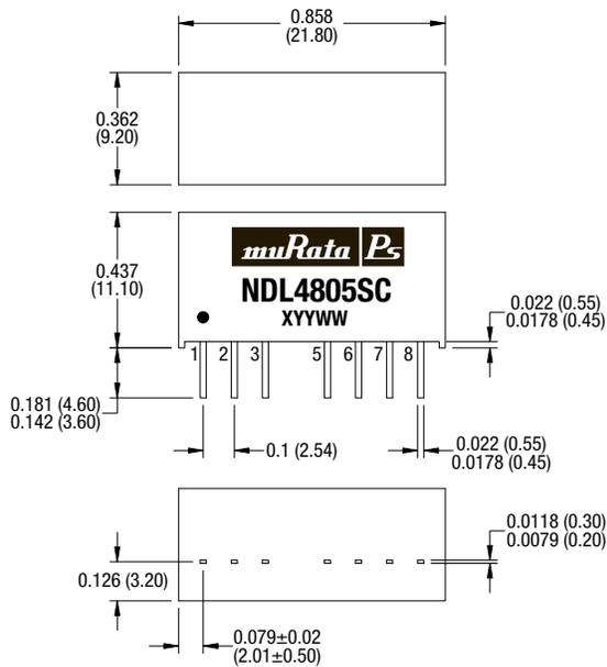
All dimensions in inches  $\pm 0.01$  (mm  $\pm 0.25$ mm). All pins on a 0.1 (2.54) pitch and within  $\pm 0.01$  (0.25) of true position. Weight: 5.0g
