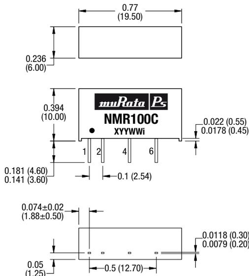
All dimensions in inches  $\pm 0.01$  (mm  $\pm 0.25$ mm). All pins on a 0.1 (2.54) pitch and within  $\pm 0.01$  (0.25) of true position. Weight: 2.1g
