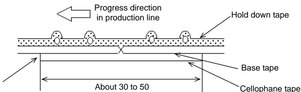
No lifting for the direction of progressing
