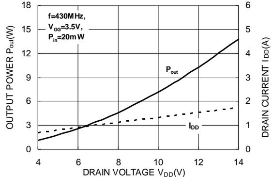
TYPICAL PERFORMANCE ( $T_{case}=+25^{\circ}C$ ,  $Z_G=Z_L=50\Omega$ , unless otherwise specified)
