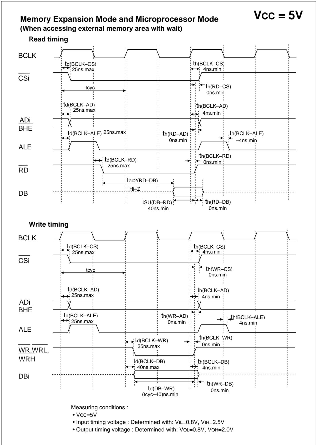
Figure 1.26.5. V<sub>CC</sub>=5V timing diagram (4)
