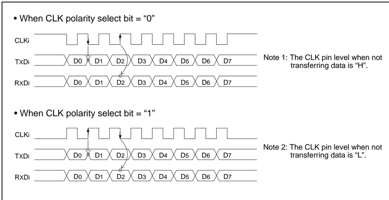
Figure 1.19.11. Polarity of transfer clock
