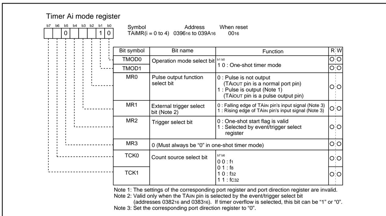
**Figure 1.17.10. Timer Ai mode register in one-shot timer mode**
