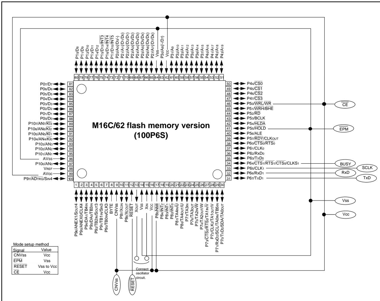
Figure 1.31.1. Pin connections for serial I/O mode (1)
