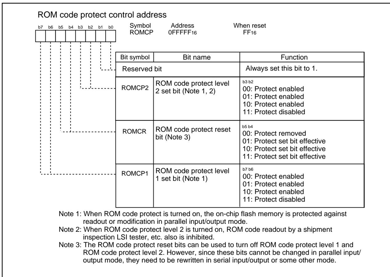
Figure 1.29.9. ROM code protect control address
