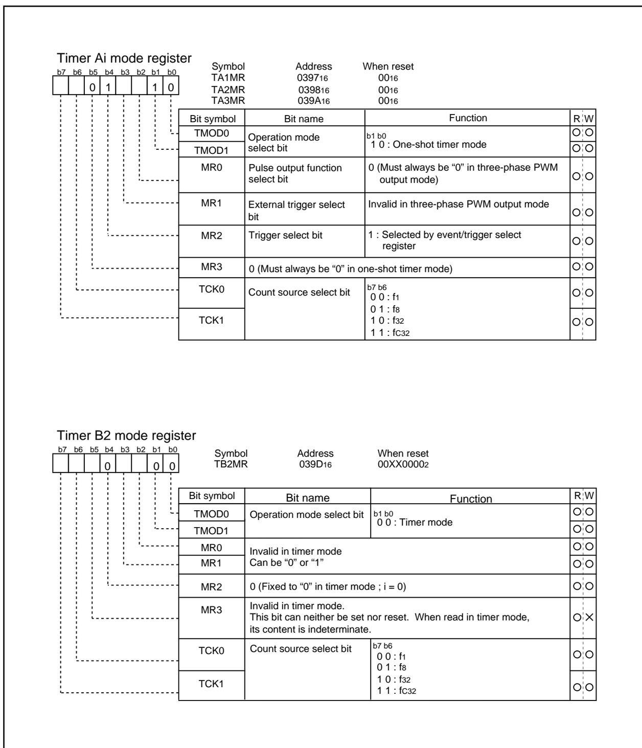
Figure 1.18.4. Timer mode registers in three-phase waveform mode
