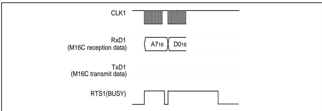
Figure 1.31.8. Timing for erasing all unlocked blocks
