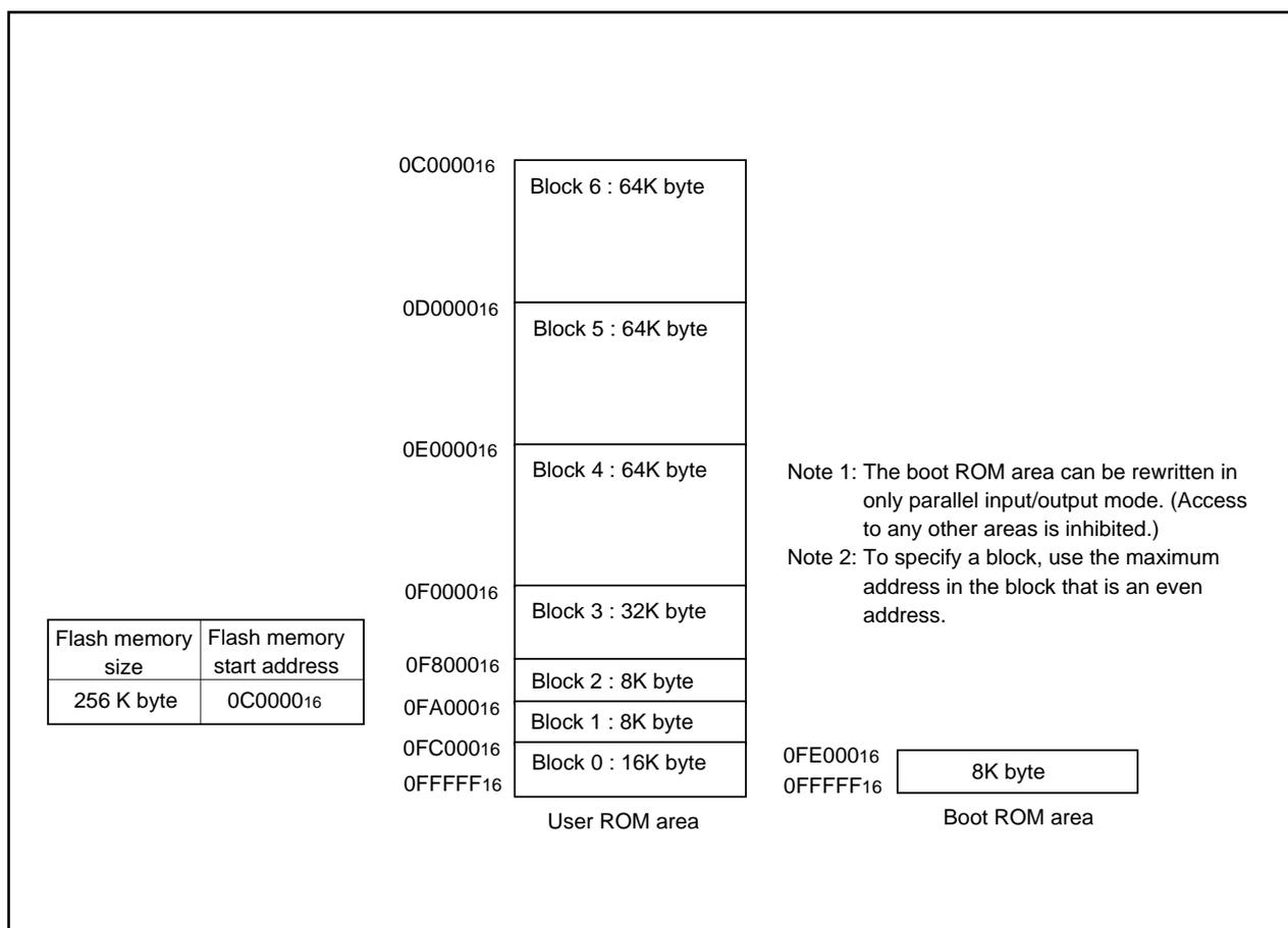
Figure 1.28.1. Block diagram of flash memory version
