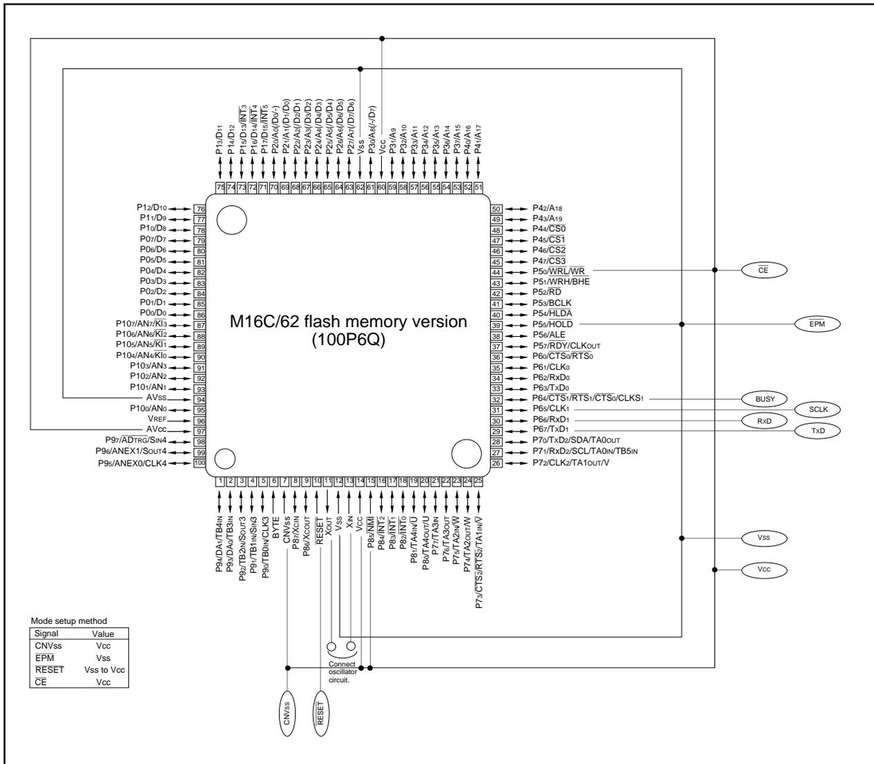
Figure 1.31.2. Pin connections for serial I/O mode (2)
