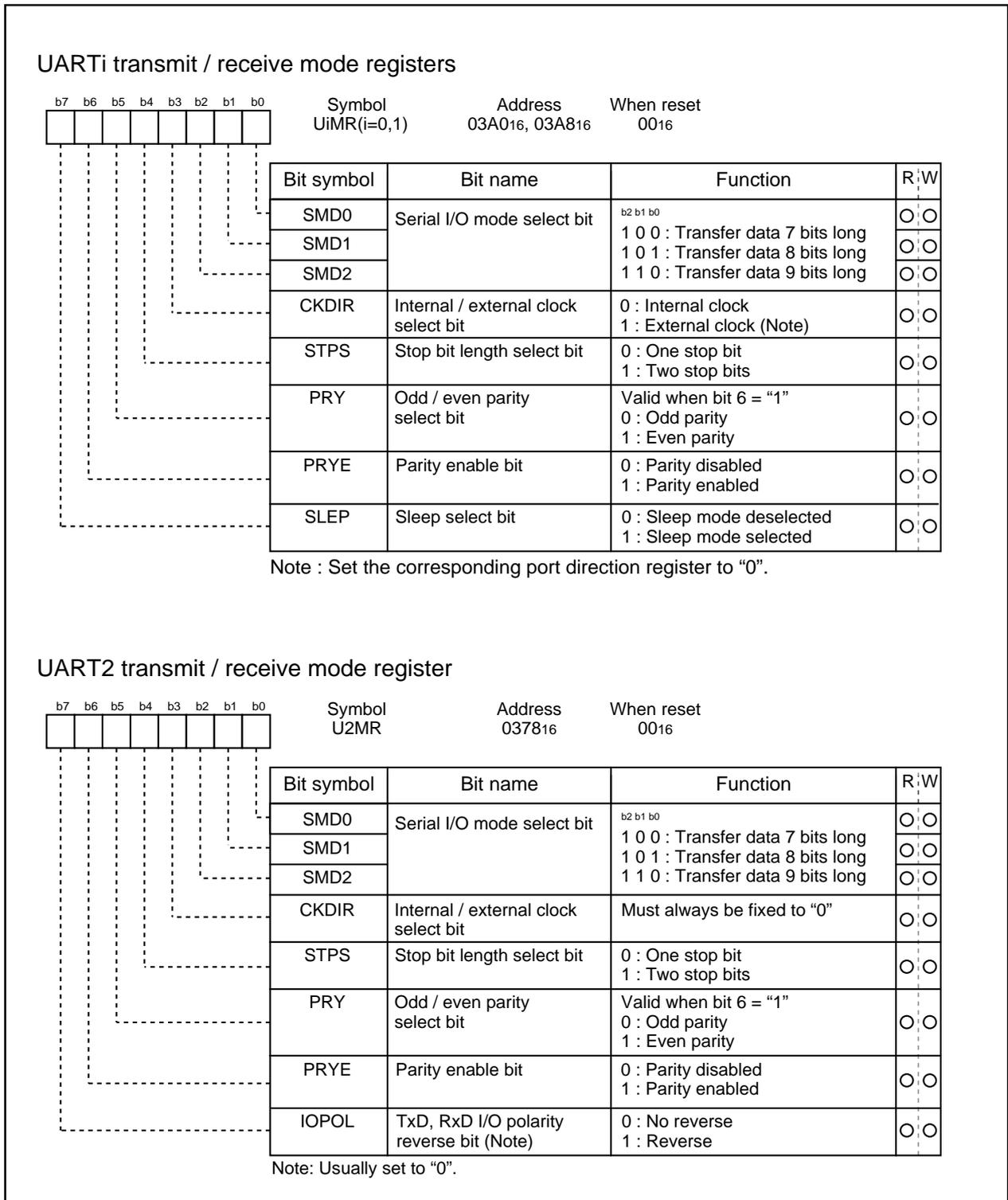
Figure 1.19.15. UARTi transmit/receive mode register in UART mode
