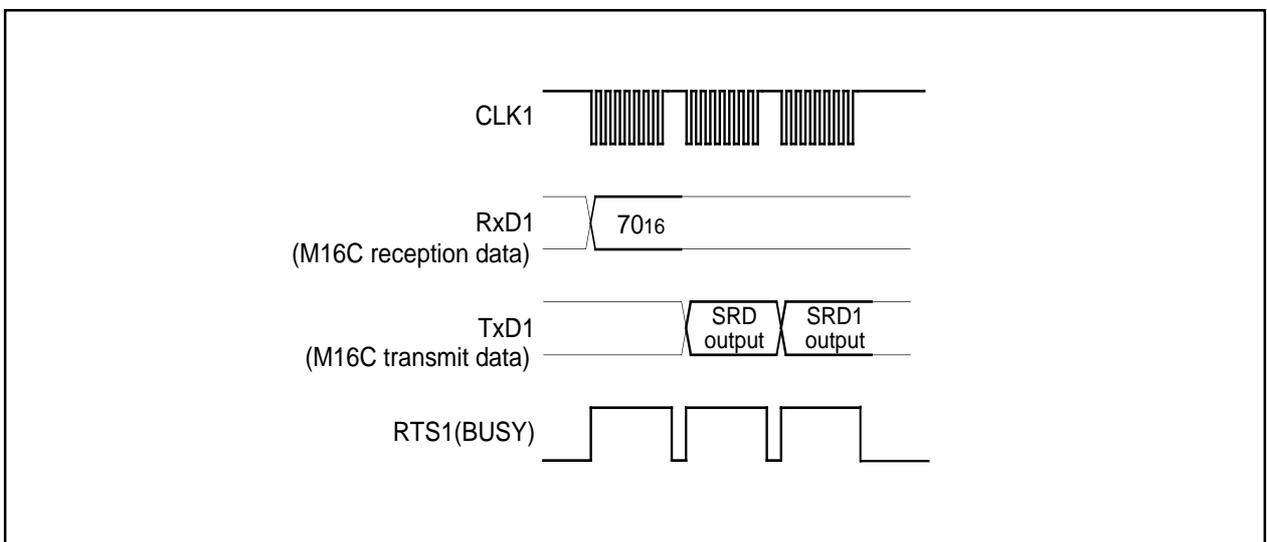
Figure 1.31.4. Timing for reading the status register
