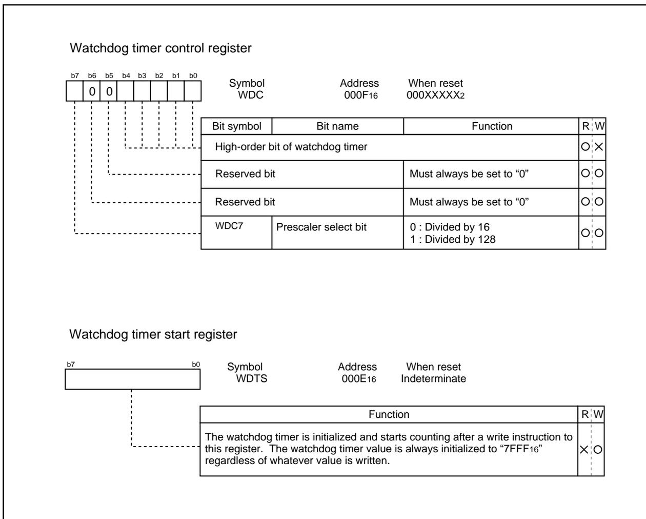
Figure 1.15.2. Watchdog timer control and start registers
