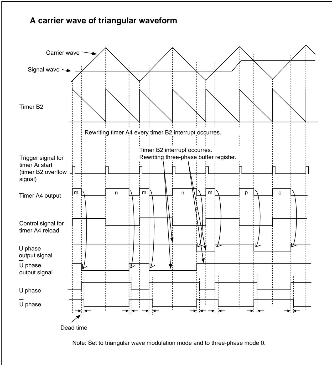
Figure 1.18.7. Timing chart of operation (2)
