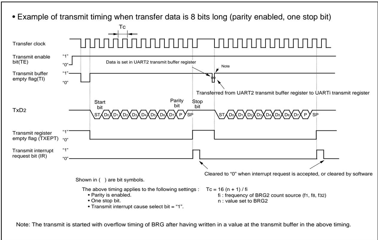
Figure 1.19.17. Typical transmit timings in UART mode(UART2)
