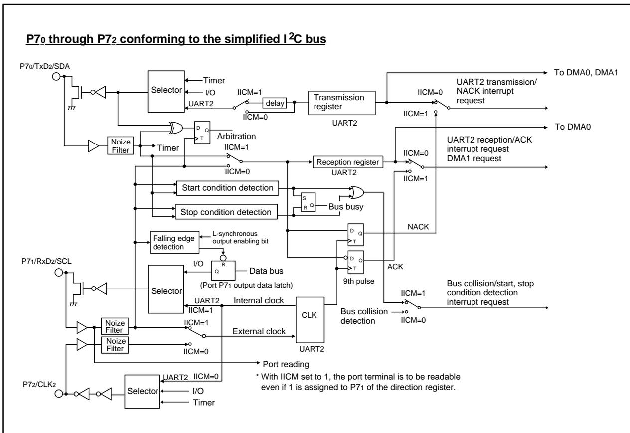
**Figure 1.19.27. Functional block diagram for I<sup>2</sup>C mode**
