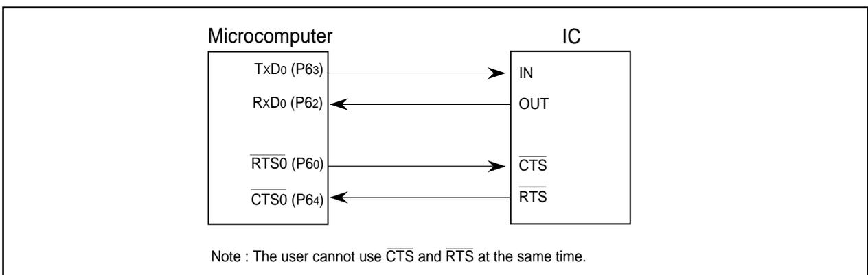
Figure 1.19.19. The separate CTS/RTS pins function usage
