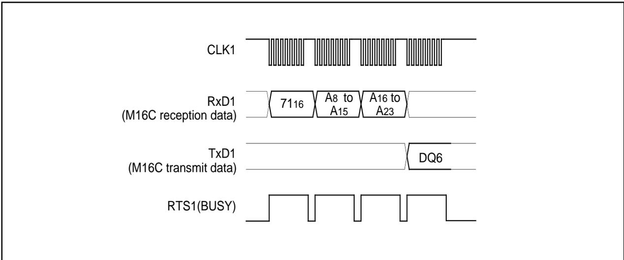
Figure 1.31.10. Timing for reading lock bit status
