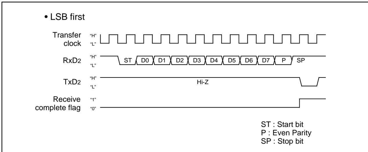
Figure 1.19.23. Output timing of the parity error signal
