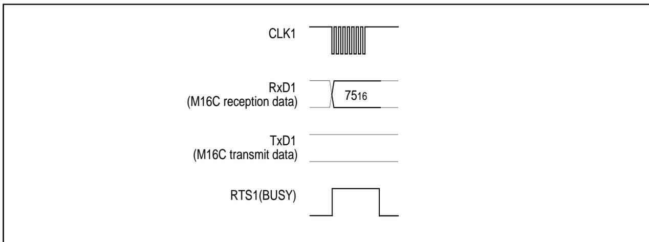
Figure 1.31.12. Timing for disabling the lock bit
