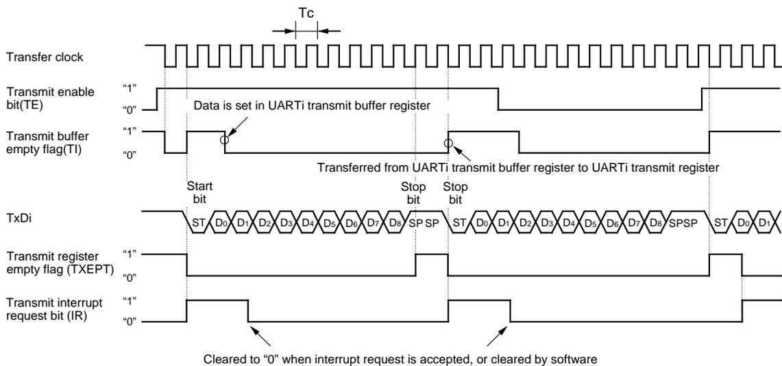
Figure 1.19.16. Typical transmit timings in UART mode(UART0,UART1)
