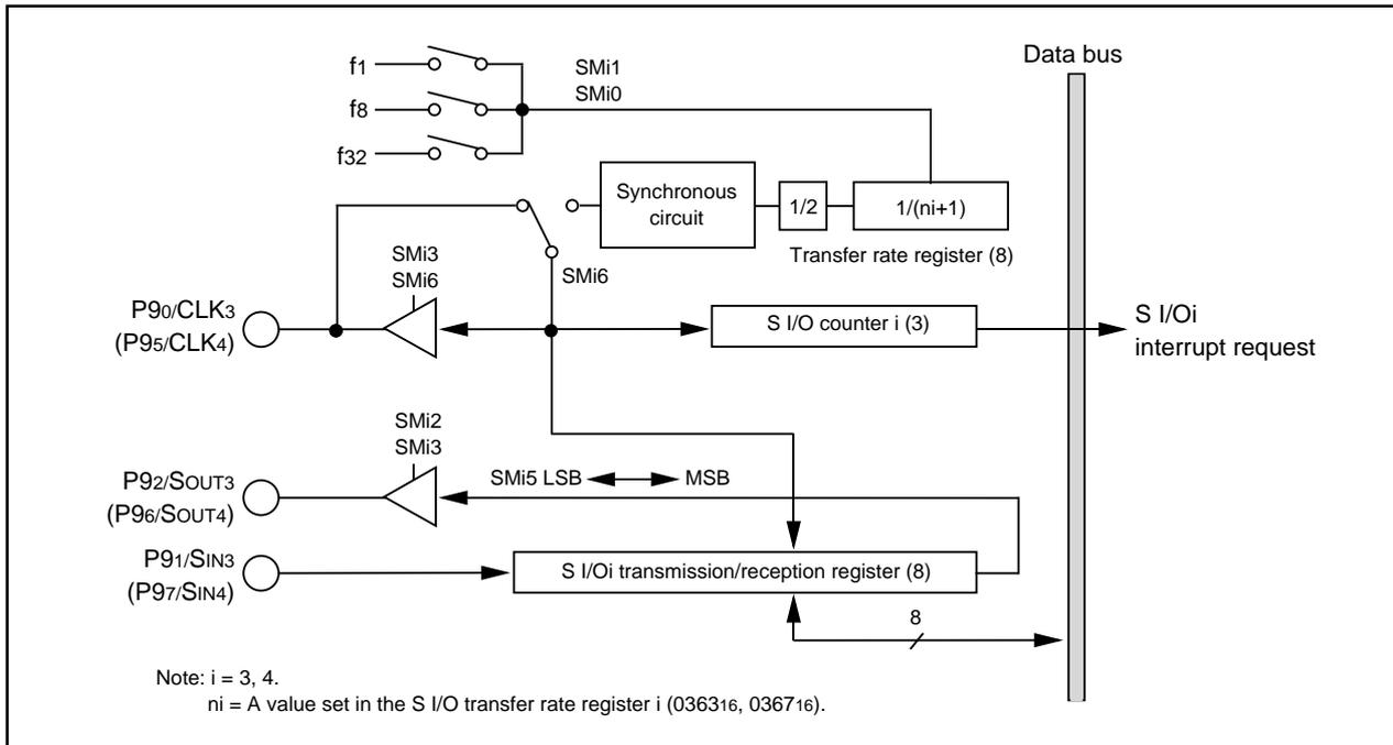
Figure 1.19.31. S I/O3, 4 block diagram
