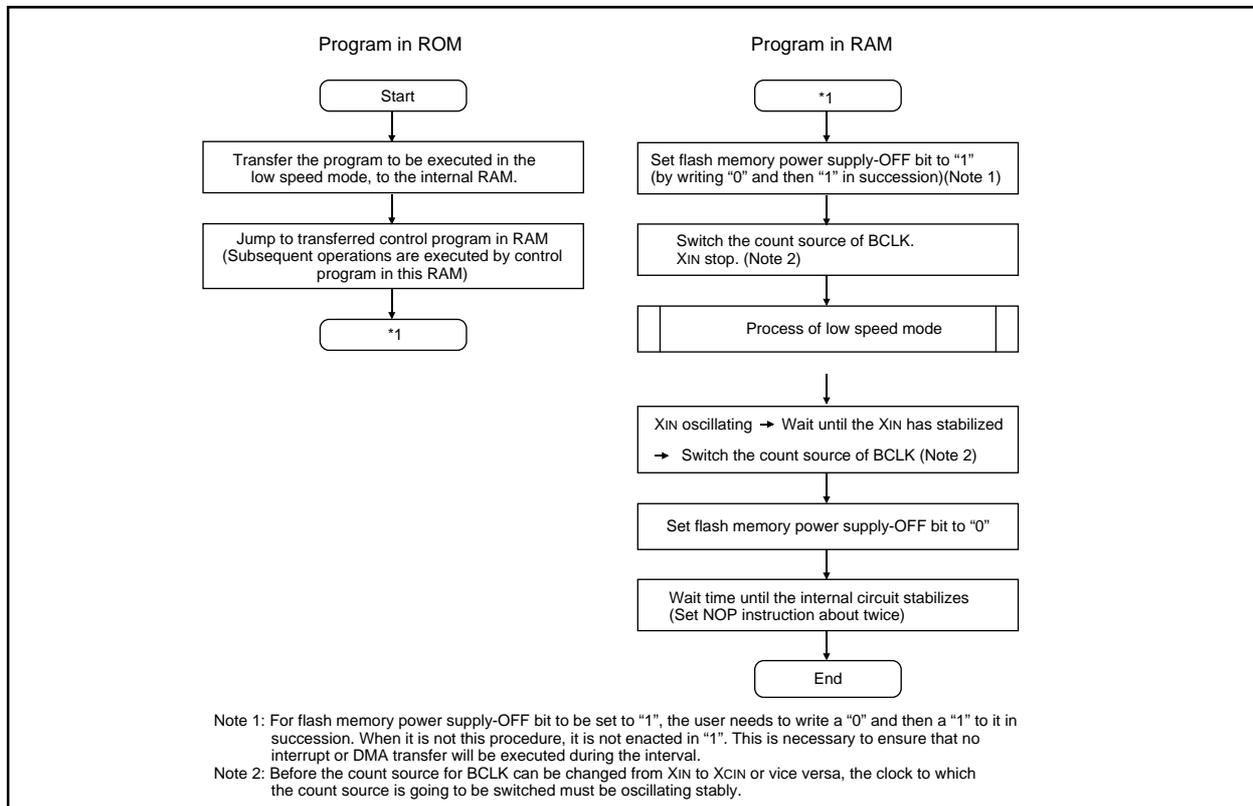
Figure 1.29.3. Shifting to The Low Speed Mode Flowchart
