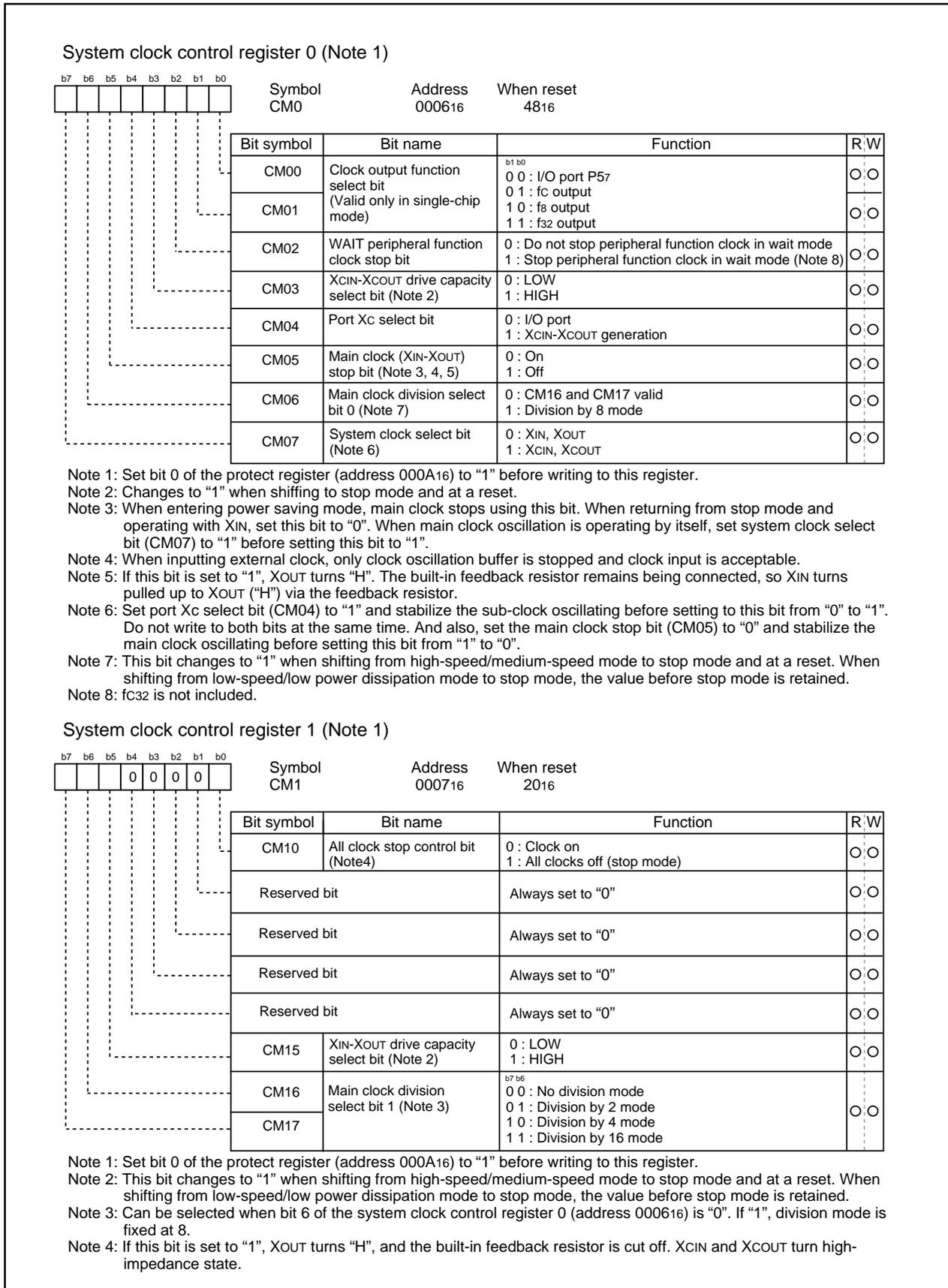
Figure 1.13.4. Clock control registers 0 and 1
