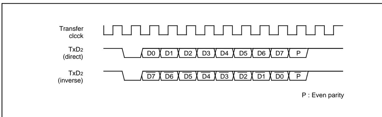
Figure 1.19.24. SIM interface format
