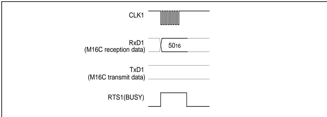
Figure 1.31.5. Timing for clearing the status register
