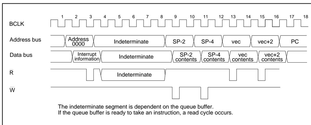
**Figure 1.14.5. Time required for executing the interrupt sequence**
