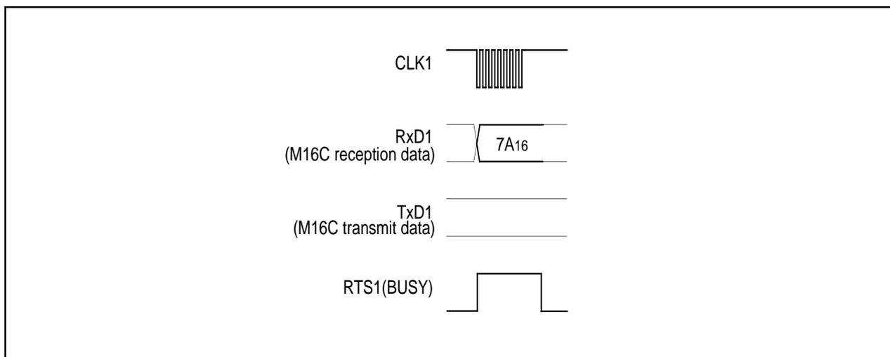
Figure 1.31.11. Timing for enabling the lock bit
