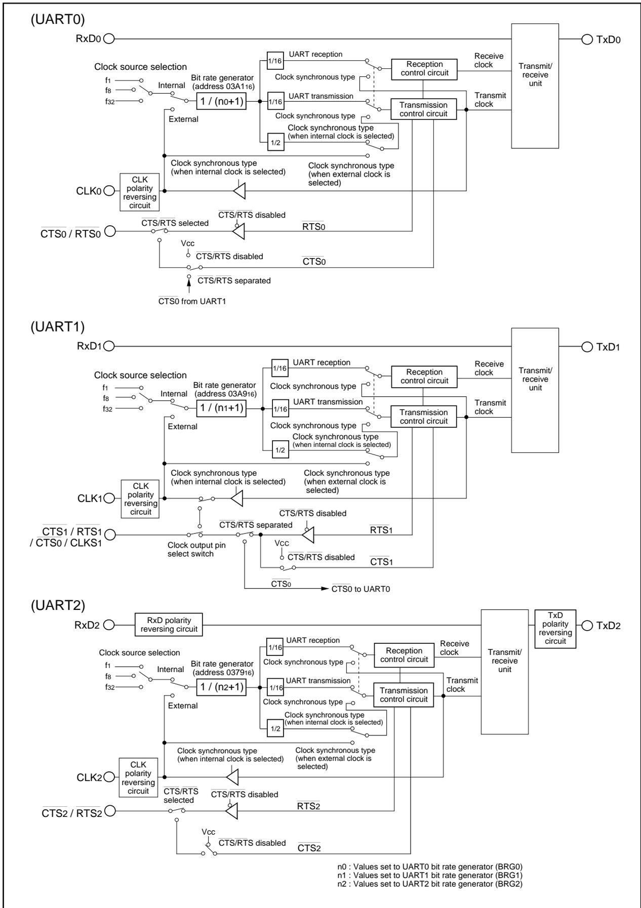
Figure 1.19.1. Block diagram of UARTi (i = 0 to 2)
