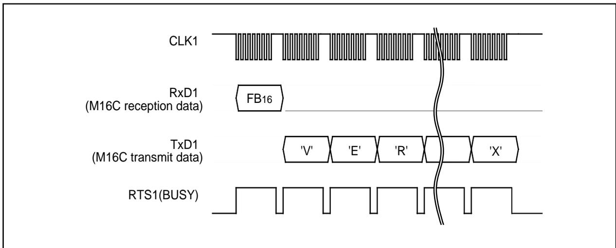
Figure 1.31.14. Timing for version information output
