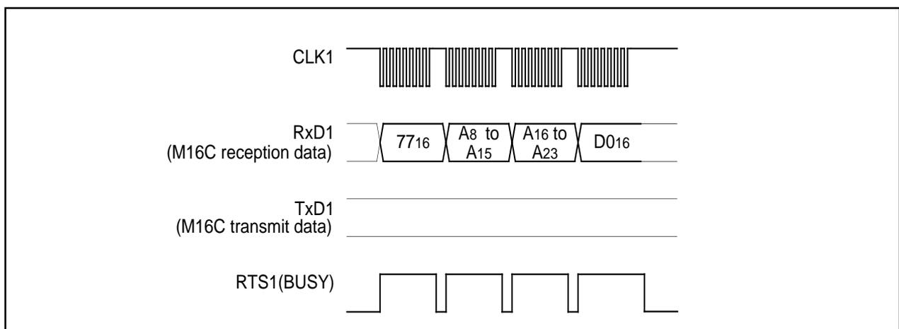
Figure 1.31.9. Timing for the lock bit program
