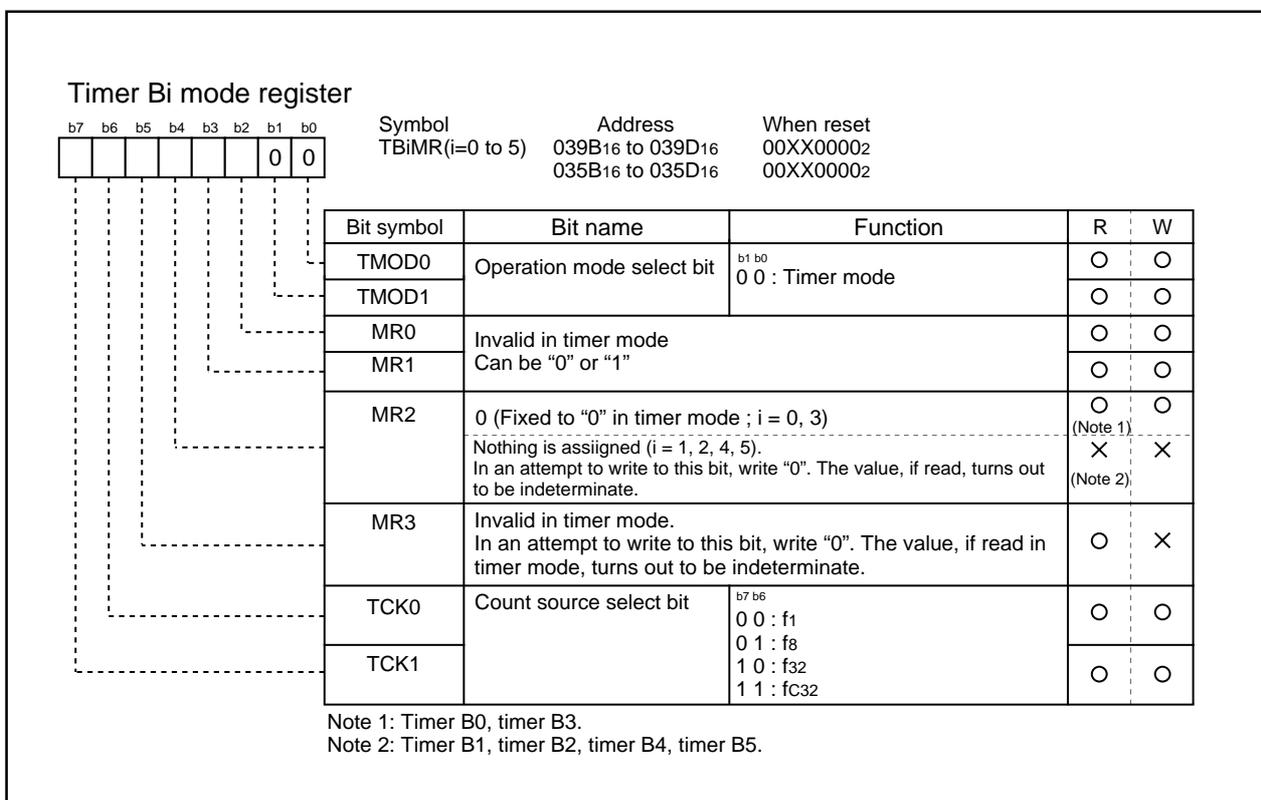
**Figure 1.17.17. Timer Bi mode register in timer mode**
