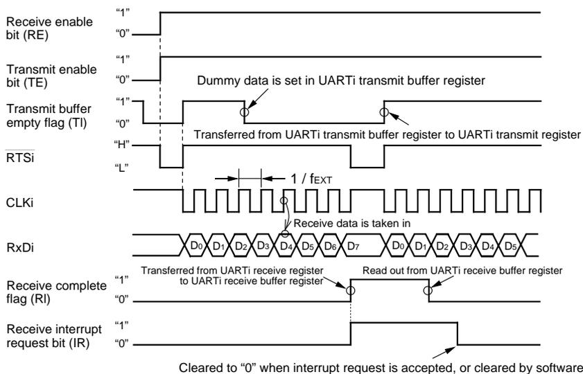
Figure 1.19.10. Typical transmit/receive timings in clock synchronous serial I/O mode
