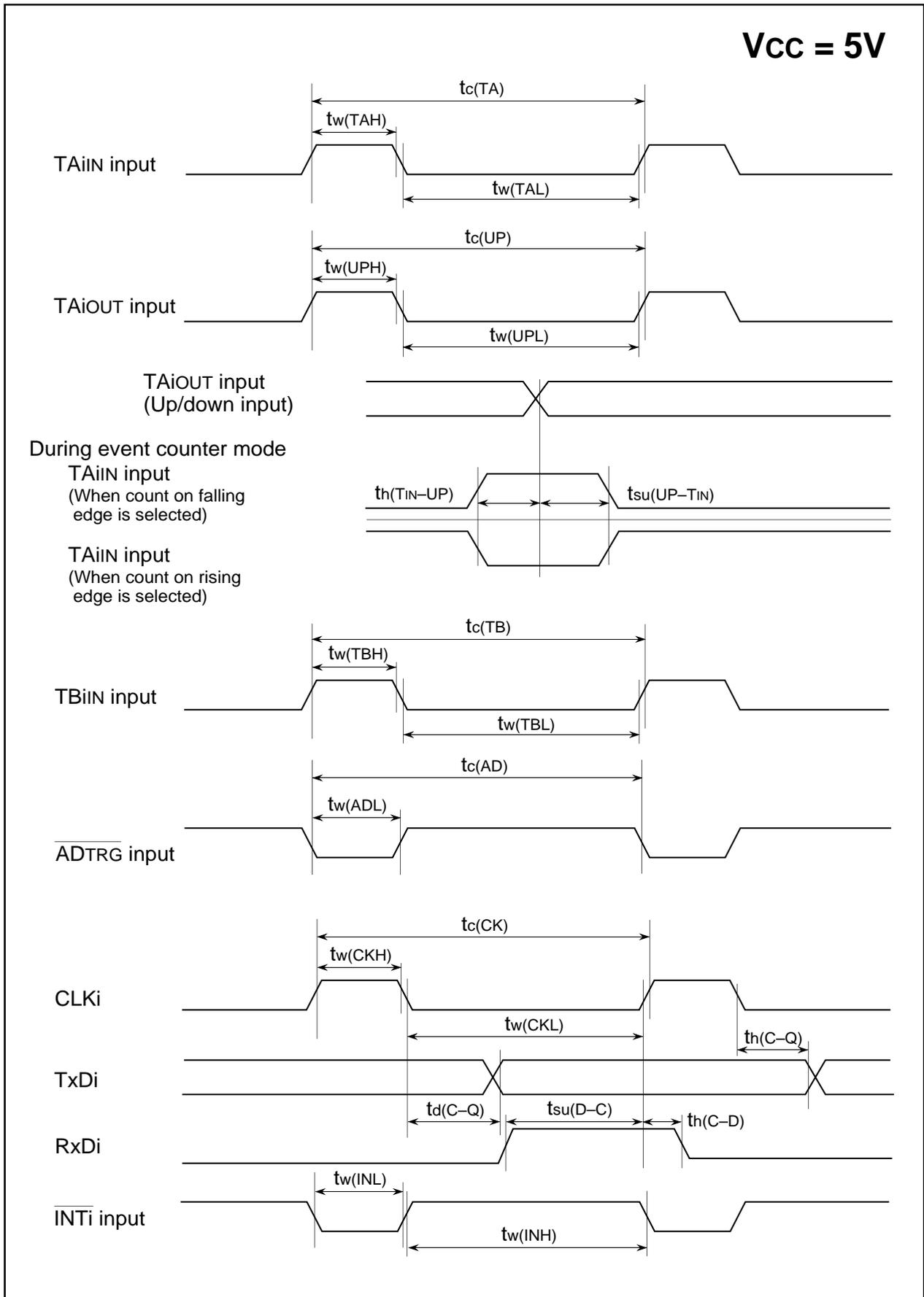
Figure 1.26.2.  $V_{CC}=5V$  timing diagram (1)
