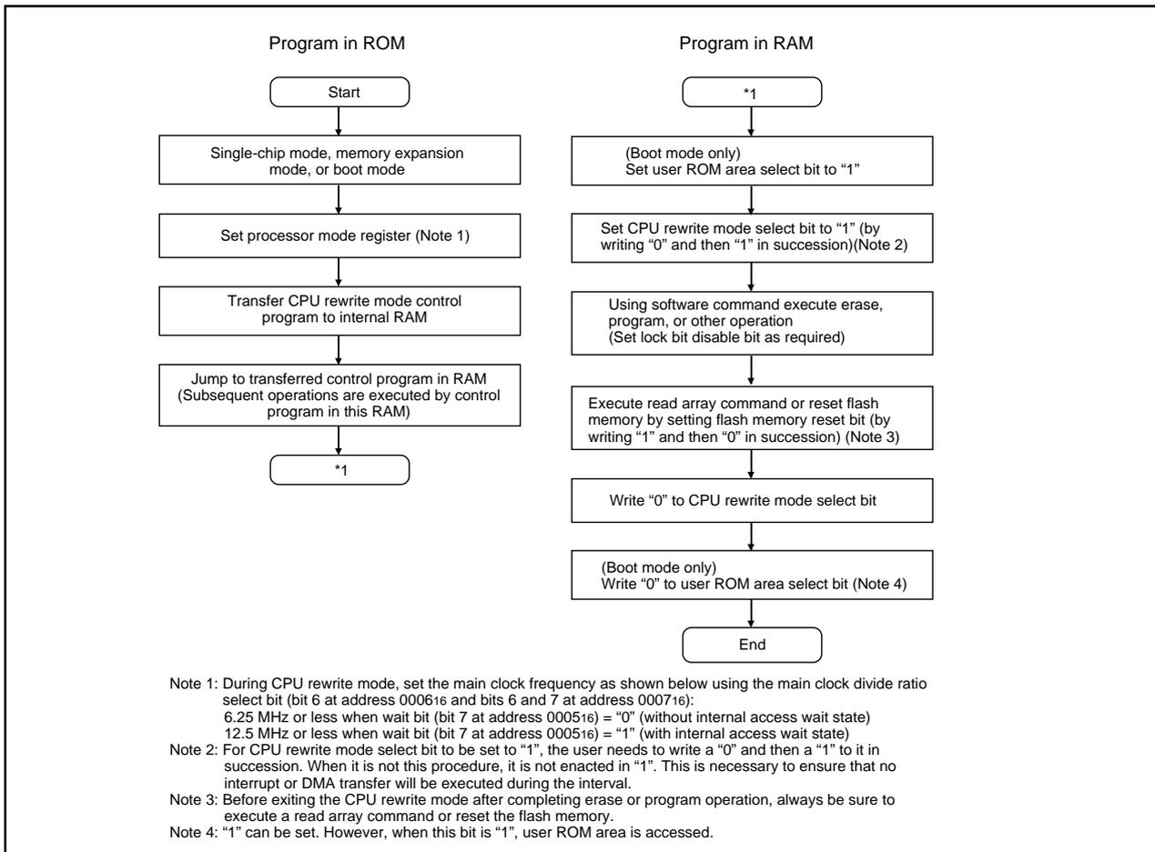
Figure 1.29.2. CPU Rewrite Mode Set/Reset Flowchart
