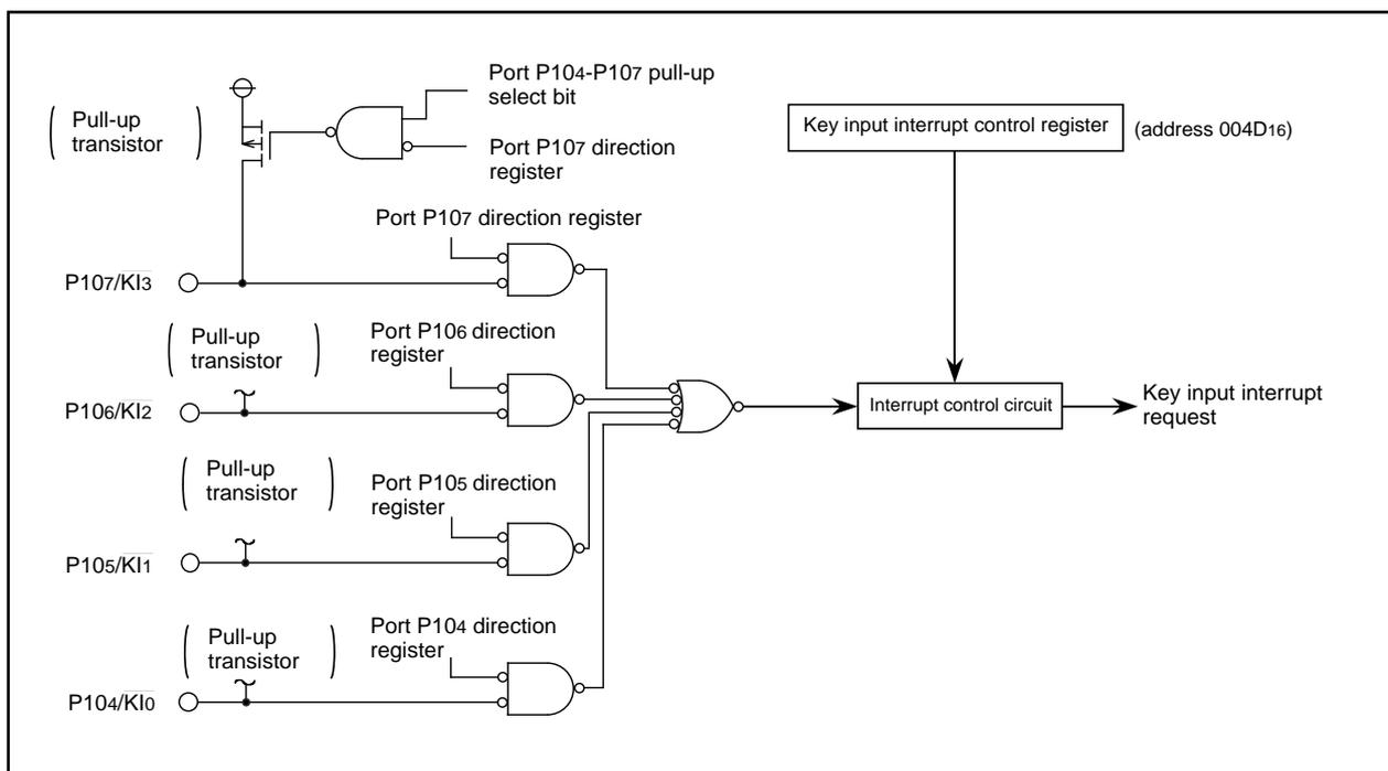
Figure 1.14.11. Block diagram of key input interrupt
