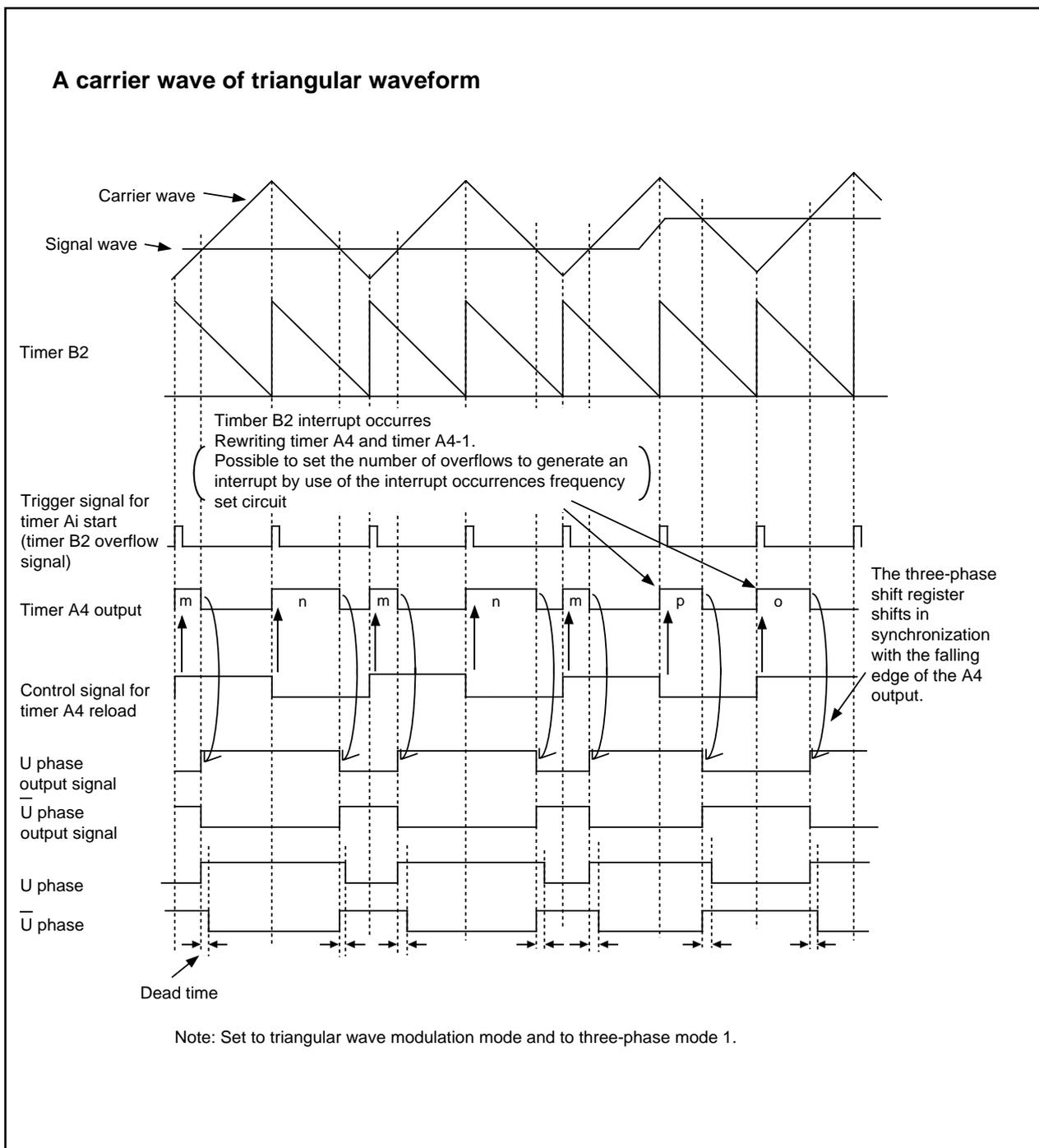
Figure 1.18.6. Timing chart of operation (1)
