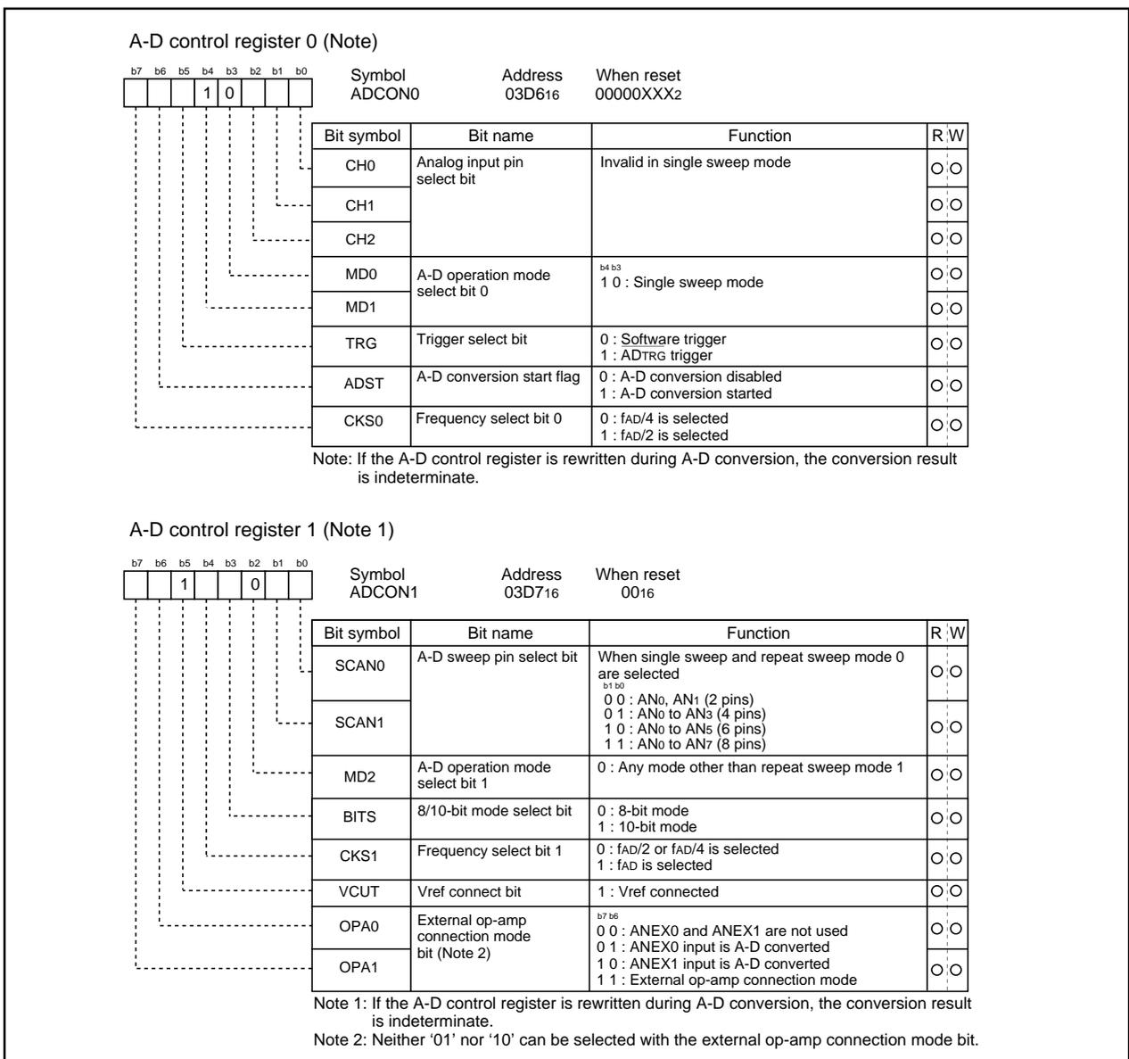
**Figure 1.20.6. A-D conversion register in single sweep mode**
